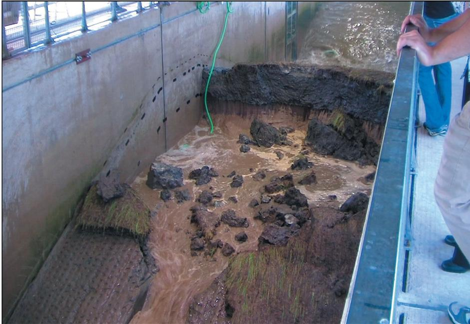
Fig. 37: Sea dike breach modelling in the GWK
