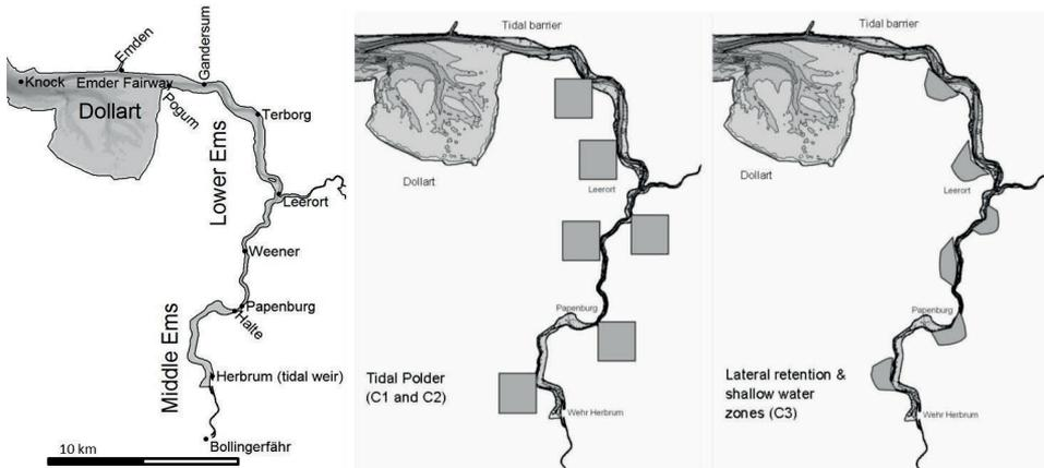
Figure 1: Overview for the Lower Ems (left), sketches of the restoration variants for the Ems Estuary, tidal polders (center) and shallow water zones (right).
