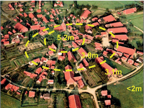
Figure 7: Dwelling mound village of Rysum in East Frisia with marker lines for existing levels above German datum; actual design water level in the area is about 6.5 m above German datum (RITZMANN and NIEMEYER 2012).
