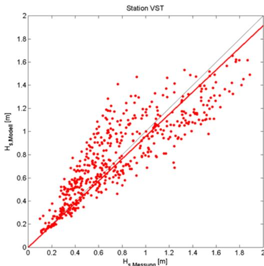
Fig. 3: Scatter plot of measured and simulated (with SWAN) significant wave heights at the station VST by Norderney (Sep.-Nov. 2002).
