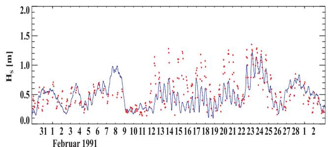
Fig. 2: Measured (red) and modelled (k-Model: blue) significant wave heights at the station Vogel-sand (Elbe estuary) in February 1991.
