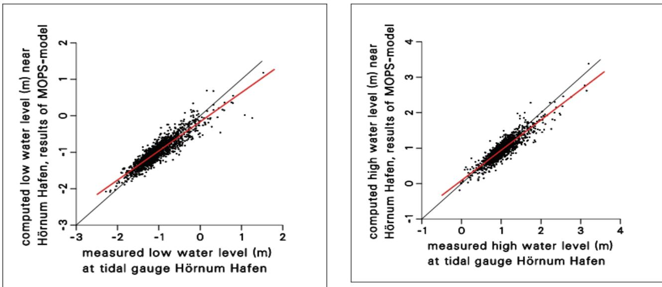
Fig. 3: Comparison of measured and simulated low water levels and high water levels at Hörnum harbour during the BELAWATT simulation period Nov 1999 – Oct 2001. The water levels refer to NN, the German ordinance level. The black lines are the  $45^\circ$  lines. The regression lines are in red.
