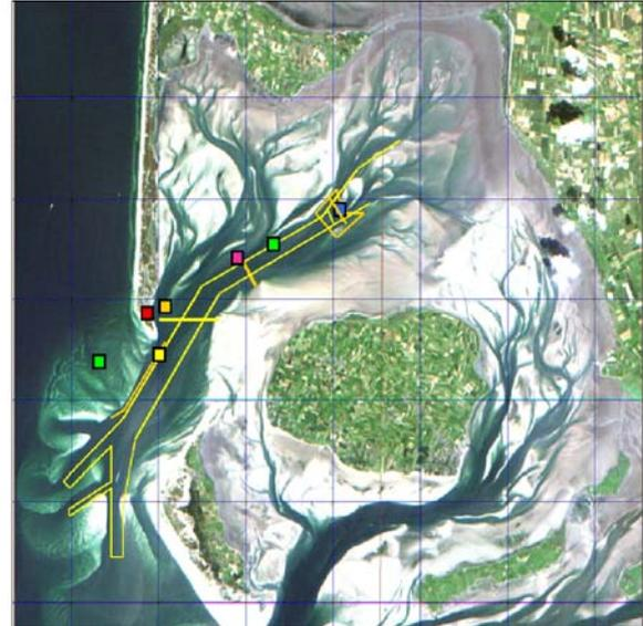
Fig. 1: The Hörnum tidal basin is located in the northern half of the map. The sites and colors of the long-term measurements: (1) monitoring pile, blue (2) bottom mounted ADCP, pink (3) wave rider buoys, green (4) WaMoS, red. The transects of the 2003 ship campaigns are shown in yellow and in orange.
