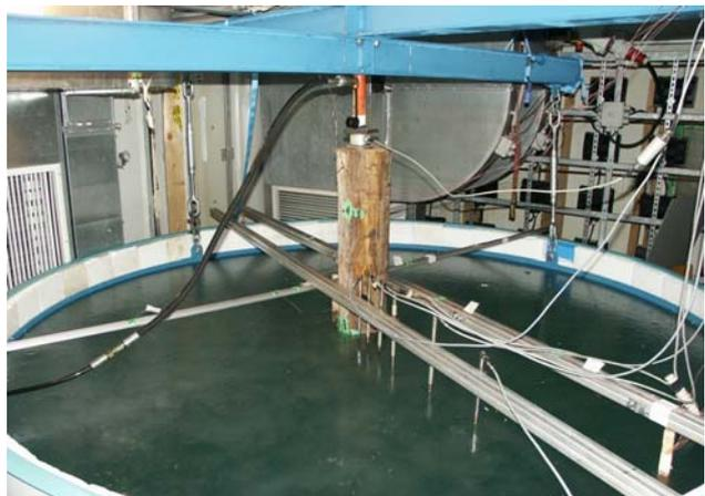
Fig. 1: Measurement of vertical ice loads in the climate chamber
