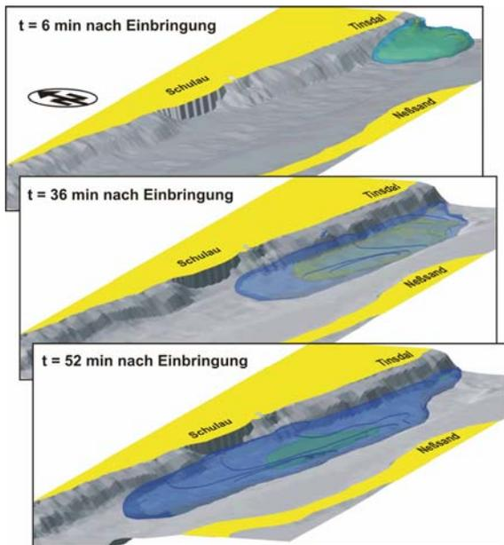
Fig. 3: Disposal induced turbidity pattern (calculated SPMC-Iso-surfaces) at three points of time.
