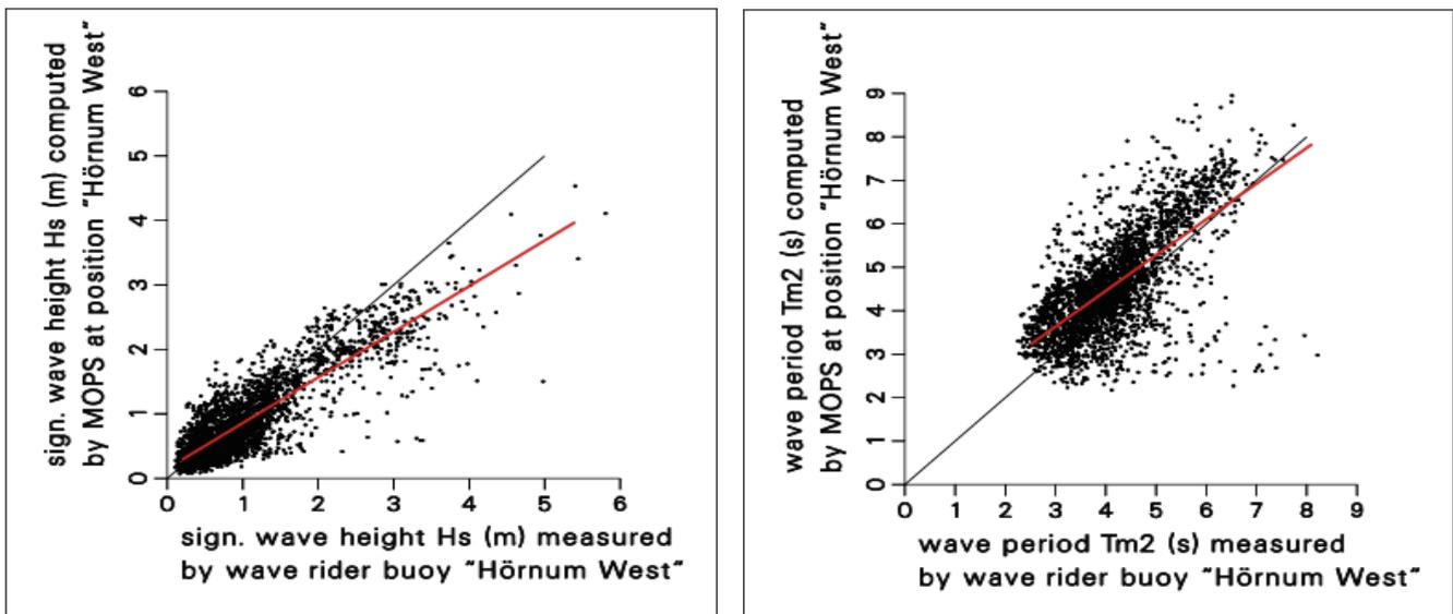
Fig. 4: Comparison of measured and simulated wave data: significant wave height  $H_s$  (left plot) and mean wave period  $T_{m2}$  (right plot). The measured data are from the wave rider buoy "Hörnum West" (see Fig. 5) of the Authority for Rural Areas in Husum. The water depth at the buoy's position is about 10 m. Period of comparison: Nov 1999 – Oct 2001. The black lines are the  $45^\circ$  lines. The regression lines are in red.
