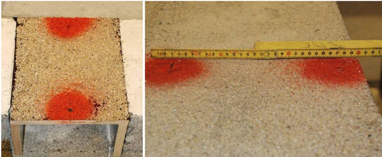
Figure 3.9 Plywood boxes and drilled holes for pressure cells
