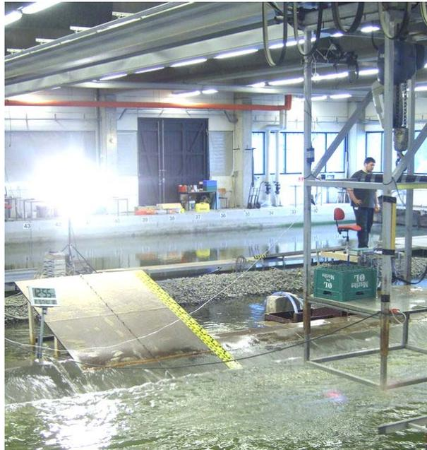
Figure 3.21 Wave run-up plate and rack with both digital cameras
