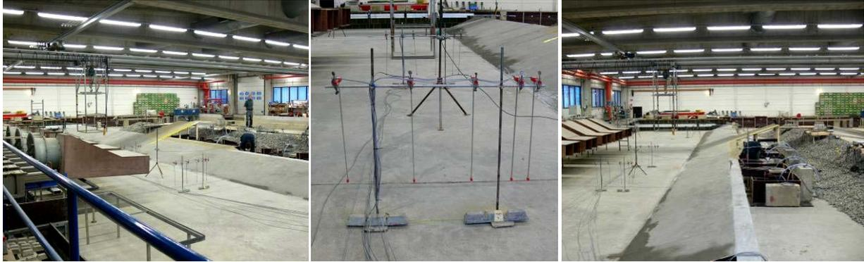
Figure 3.12 Overview of the basin: Wind machines; Wave array, Anemometer; Dike and overtopping unities
