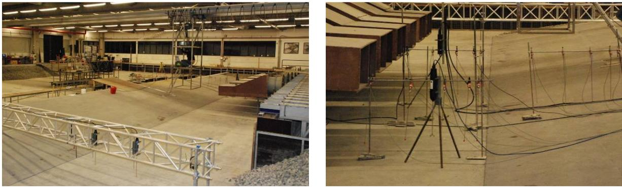
Figure 3.8 View from the upstream inlet of the 1:6 dike setup, wind machines and wave gauges in front of the dike
