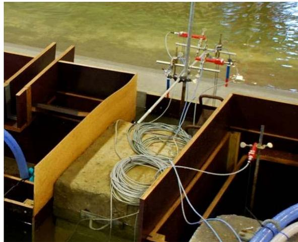
Figure 3.28 Overtopping boxes with channel and measurement devices for flow depth and flow velocity measurements
