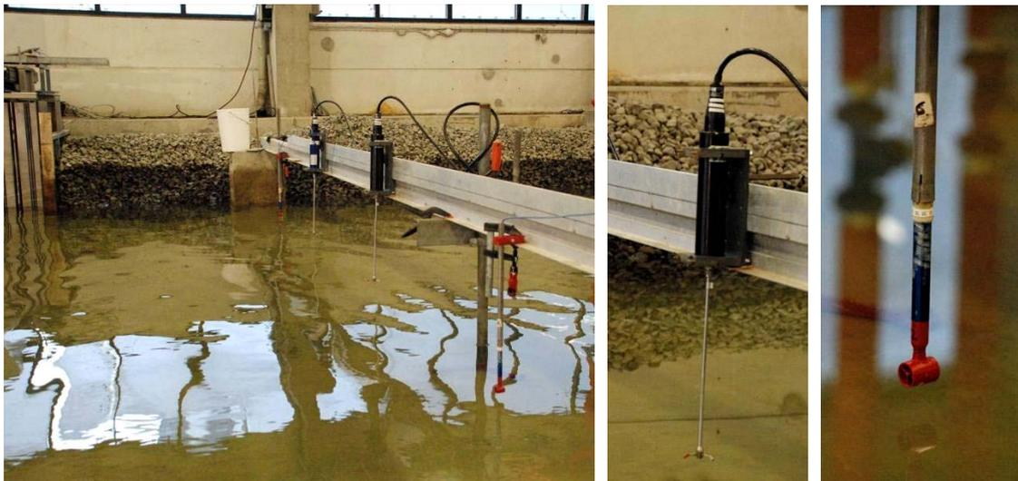
Figure 3.19 Beam upstream the wave machine; ADV; Micro propeller (FlowDike 1)
