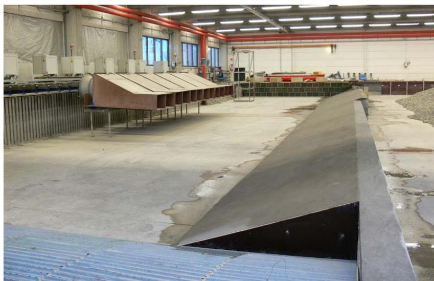
Figure 3.1 Completed dike slope (view from downstream), wave generator (paddles) and wind generator (fans) on the left side.
