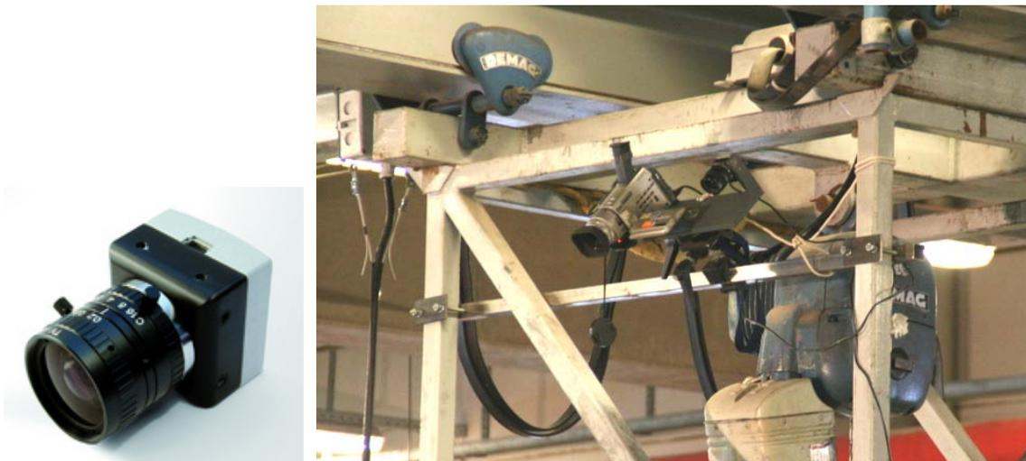
Figure 3.24: Left: USB-camera, Right: Both cameras mounted on a rack in the model setup
