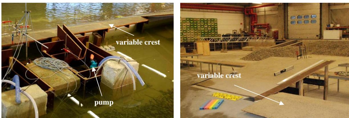
Figure 3.4 Overtopping boxes in front of the variable crest (left); Run-up board and variable crest during construction (right)
