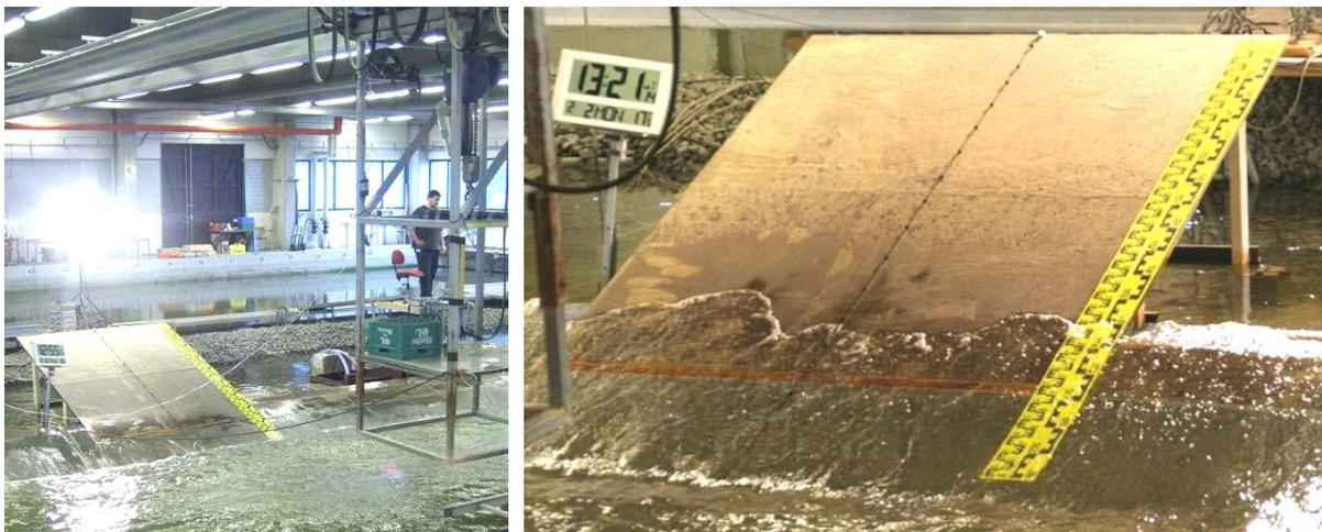
Figure 3.6 Wave run-up plate and rack with both digital cameras (left); Capacitive gauge, clock and scale (right)
