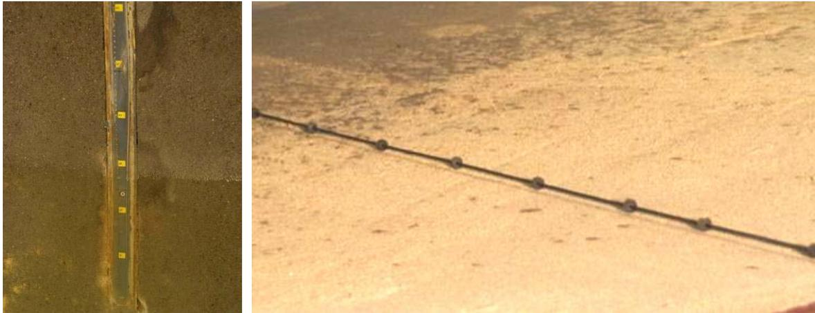
Figure 3.7 Digital step gauge within the 70 cm slope (left); Capacitive wave run-up gauge on the dike slope (right)
