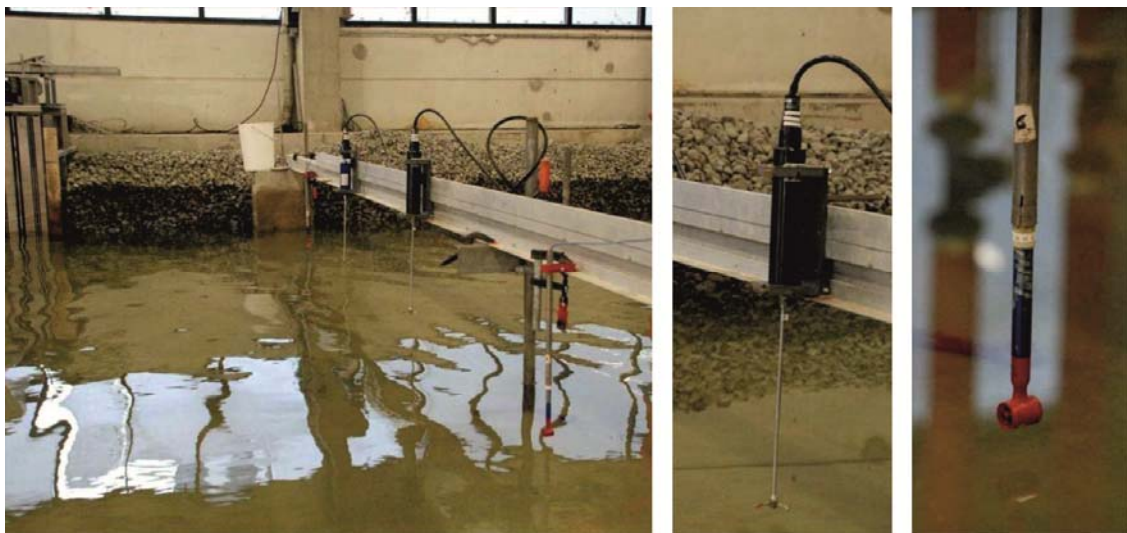
Figure 3.15 Beam upstream the wave machine (on the left side), flow direction from right to left; ADV; Micro propeller (FlowDike 1)
