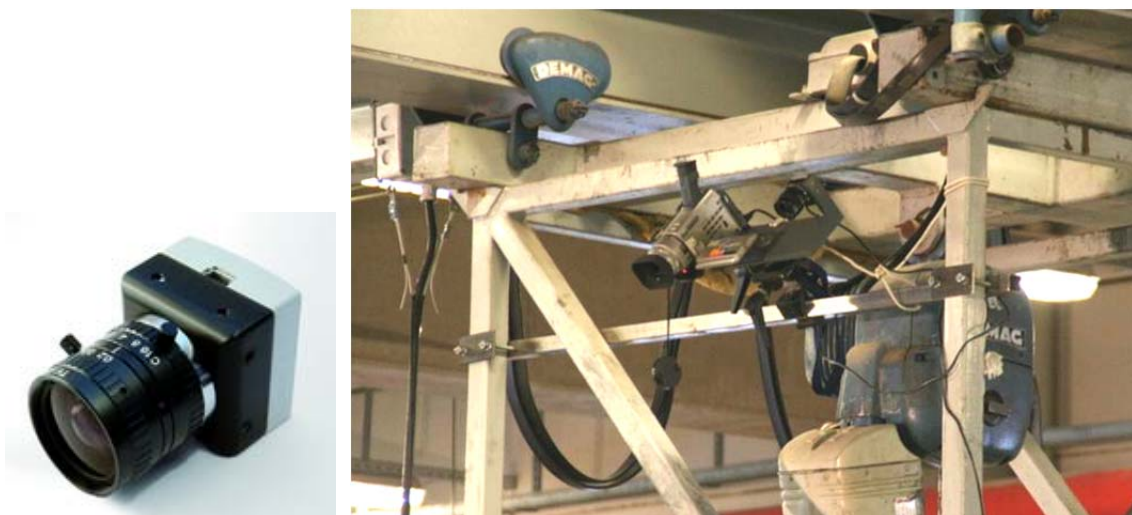
Figure 3.20: Left: USB-camera, Right: Both cameras mounted on a rack in the FlowDike 1 model set-up
