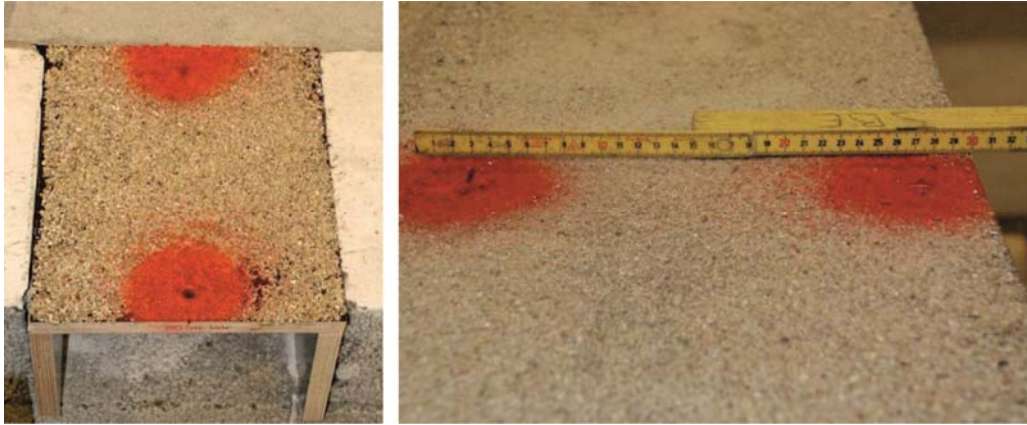
Figure 3.24 Plywood boxes and drilled holes for pressure sensors
