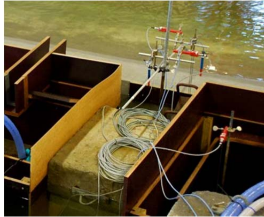
Figure 3.26 Overtopping units with channel and measurement devices for flow depth and flow velocity measurements
