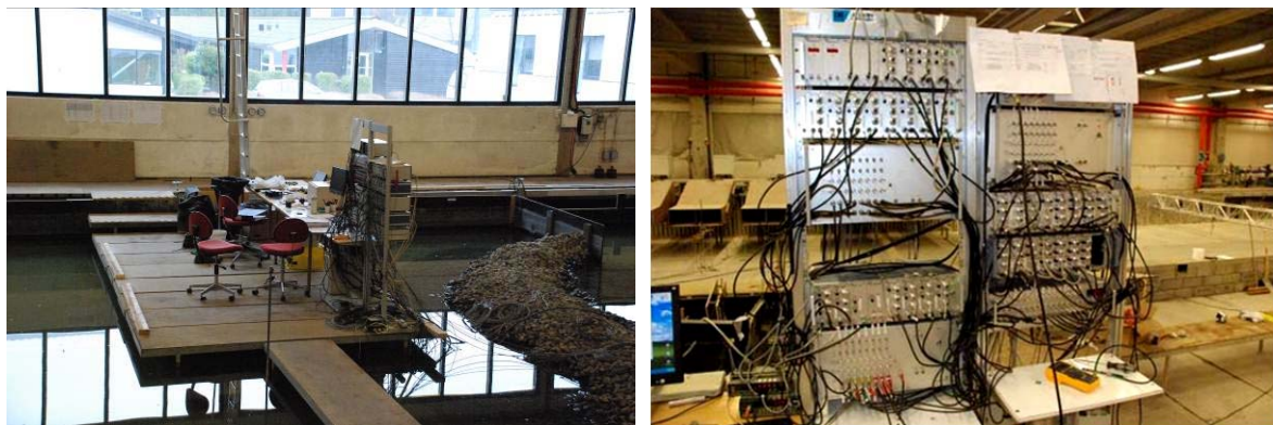
Figure 3.3 Platform with data acquisition; Stand with amplifier and A/D converter
