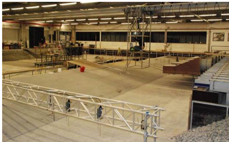
Figure 3.7 View from the upstream inlet of the 1:6 sloped dike set-up, wind machines and wave gauges in front of the dike
