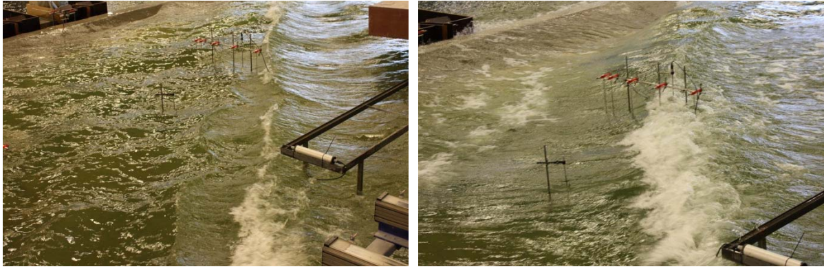
Figure 7.9 Beginning of breaker process of waves (wave propagation from right to left)
