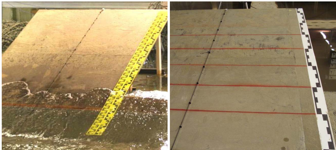
Figure 3.18: Capacitive gauge and visual gauge on the run-up board (left: FlowDike 1, right: FlowDike 2).
