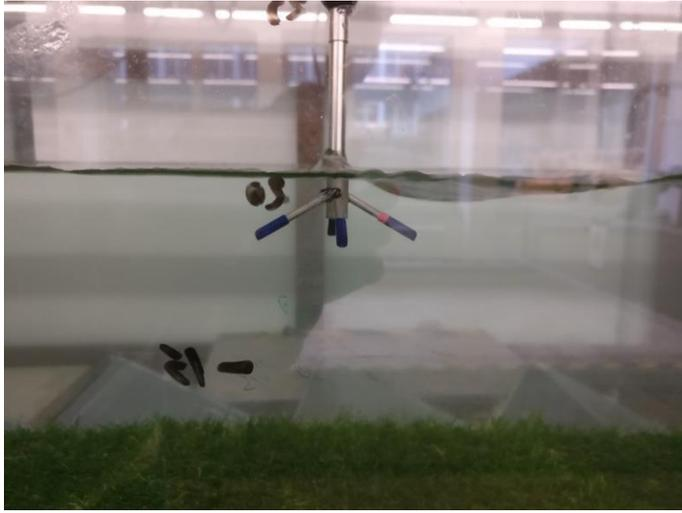
Figure 3.10. Four-beam down-looking probe of the ADV Vectrino Profiler interacting with the free surface. Note the wake occurring downstream of the probe, resulting in a trough that can eventually trap air (flow from left to right).
