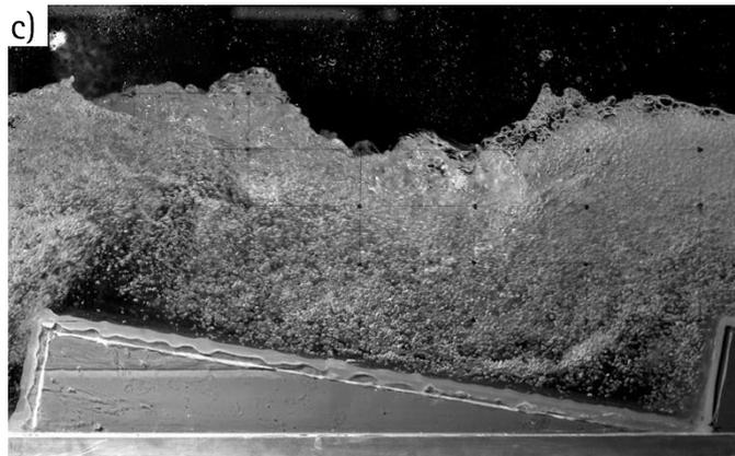
Figure 3.3. Air-water flow over the different studied models: a) 1V:2H\_AW, b) 1V:3H\_AW and c) 1V:6H\_AW. Images obtained with the high-speed camera (flow from left to right).
