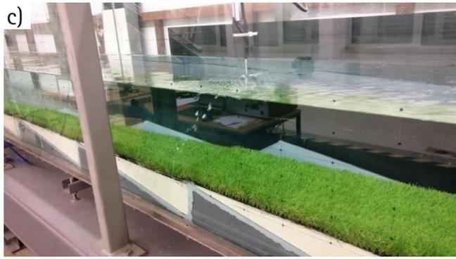
Figure 3.4. Flow over the different studied models with grass over the stepped edges: a) 1V:2H\_GE, b) 1V:3H\_GE and c) 1V:6H\_GE (flow from left to right).
