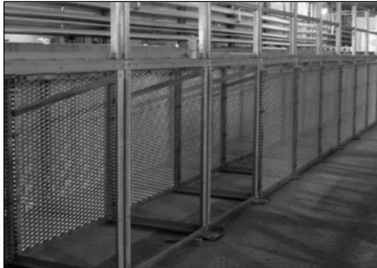
Figure 22: Side view of the passive wave absorbers
