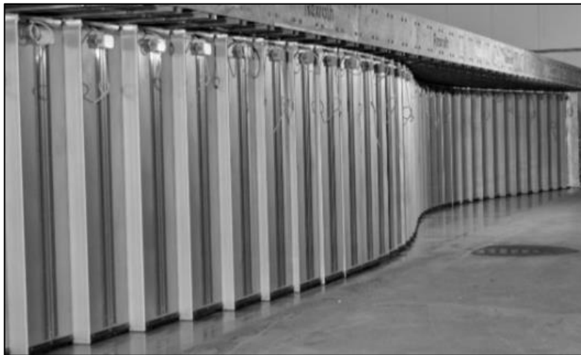
Figure 21: The installed wave generator inside the wave basin in 2011.
