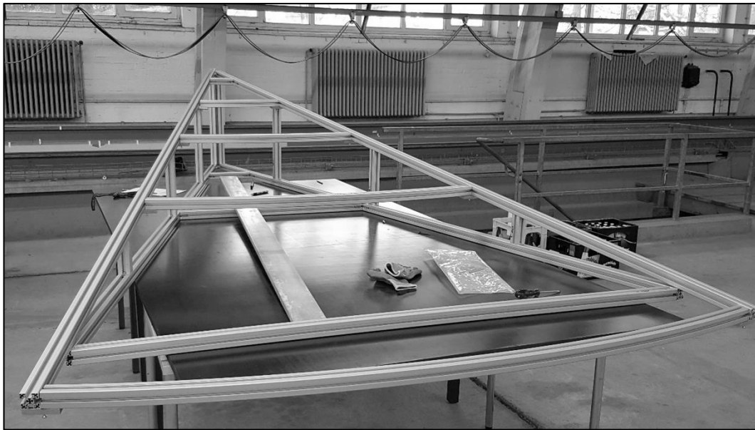
Figure 17: A single aluminium frame of a convex dike segment with curved crossbars.
