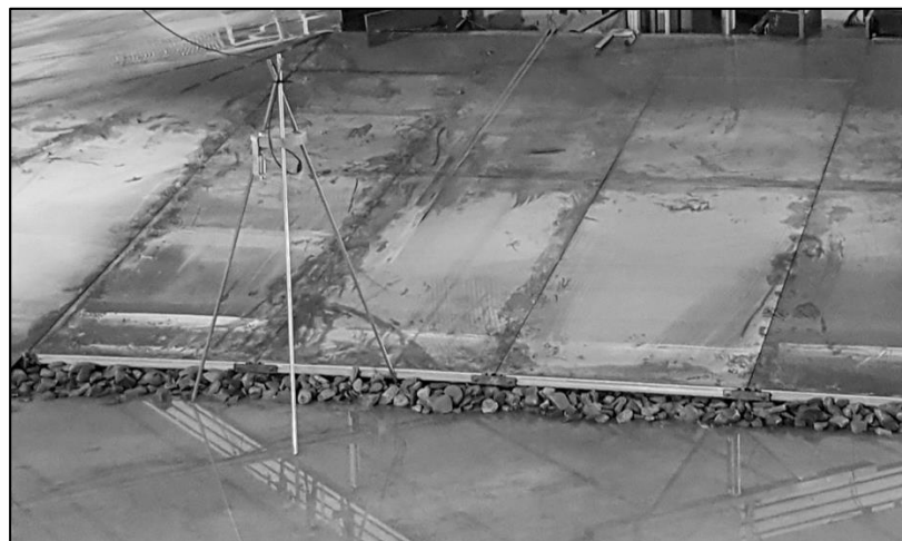
Figure 37: Sealing of the dike's front with stones and tripod with a wave gauge.
