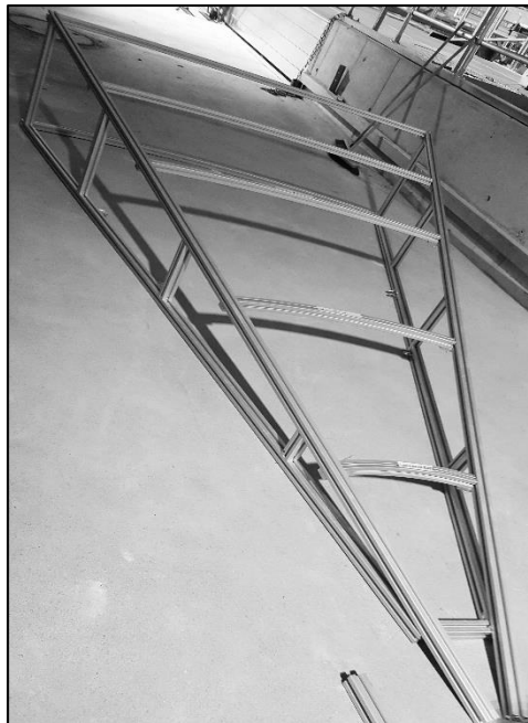
Figure 19: Bare aluminium frame of a concave dike segment with curved crossbars.
