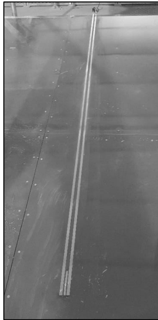
Figure 25: Integrated run-up gauges on the reference dike
