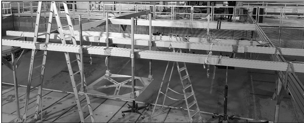
Figure 38: Measurement instruments (ea. CERC-6 wave array) were fixed to metal crossbeams.
