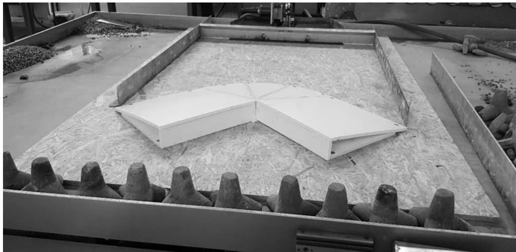
Figure 9: Model set-up of the scaled-down dike (1:10) in the small wave basin.
