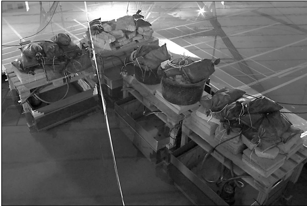
Figure 29: Weights placed on top of the overtopping units.
