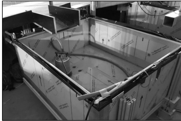
Figure 27: Overtopping unit with channel and pump.
