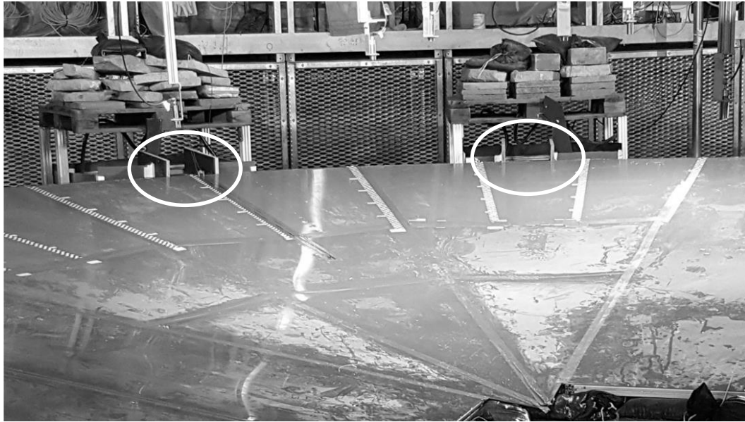
Figure 50: Overtopping inlet channels at a concave corner.
