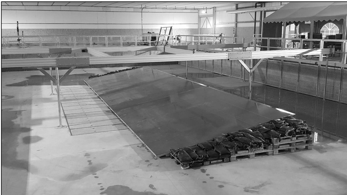
Figure 39: Reference dike with wave absorbers on the sides. On this picture, the measurement devices and cameras are not yet mounted and the front of the dike is not yet sealed.
