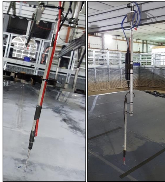
Figure 26: Vectrino Plus sensors (No. 1 left, No. 2 right) installed in the basin. The red tubes carry the aluminium oxide solution.
