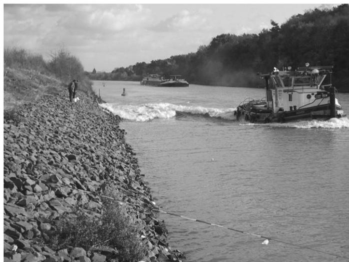
*Figure 5.14 Slope supply flow for vessels sailing close to a bank. The photos show a laden inland cargo vessel (GMS) (top), an empty inland cargo vessel (GMS) (centre) and a tug boat (bottom) in a standard trapezoidal profile (T-profile)*
