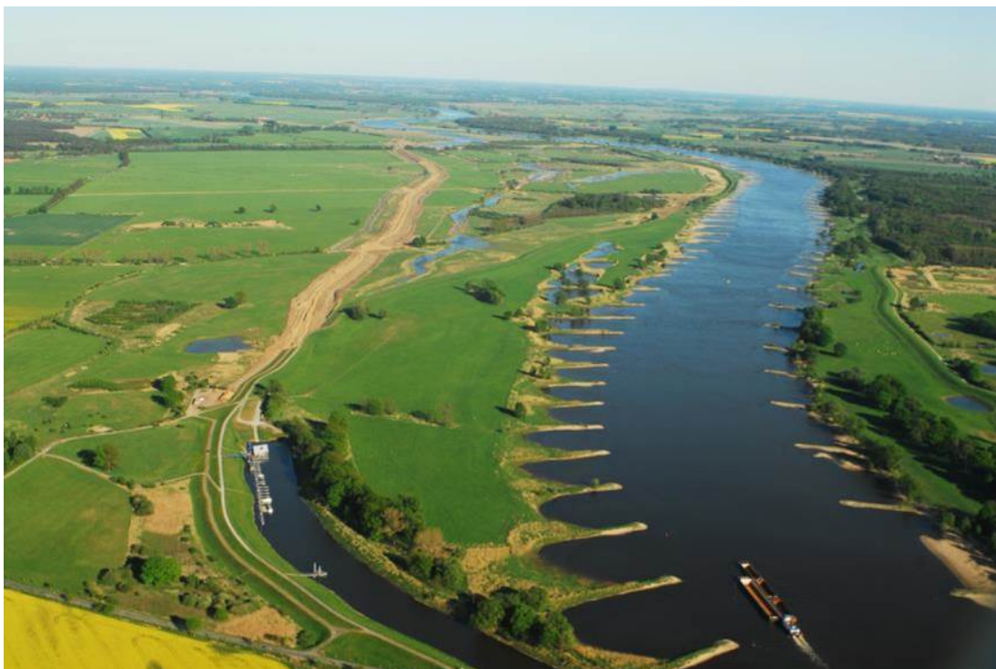
Figure 8.2 – Picture of Elbe river, looking upstream from the harbour of Lenzen – Construction phase of the dike relocation (picture taken by J.Purps, 2007-04-29)
