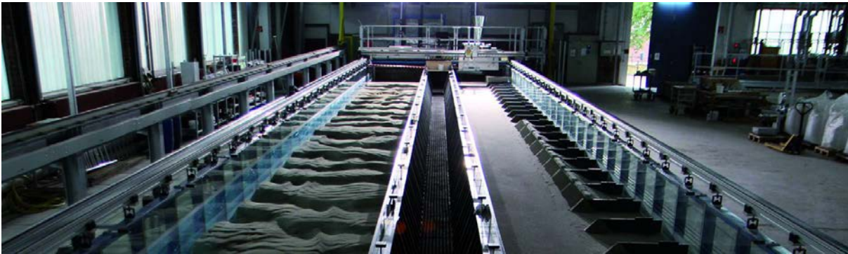
Figure 3.1 – Experimental flume for morphodynamic experiments at the Federal Waterways Engineering and Research Institute in Karlsruhe (source: BAW Bildarchiv)
