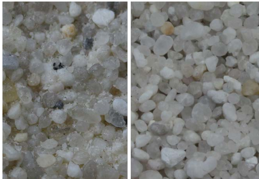
Figure 3.5 – Fixed (left) and unfixed sand in the experimental flume (LWI, 2012b)
