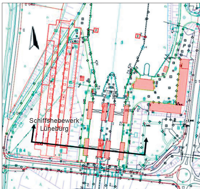
Bild 5: Lageplan SHW Lüneburg und geplante Schleuse einschl. Schnittführung 2D-FEM-Untersuchung Figure 5: Site plan of the ship lift and planned lock including profile for the preliminary 2d finite element simulation
