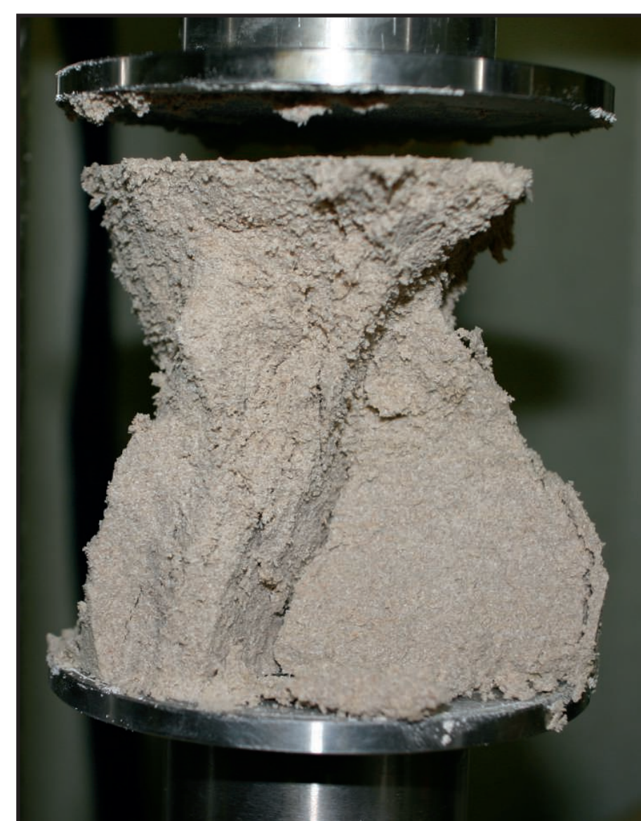
Unconfined compression test at a fully disintegrated sandstone (FG 1)
