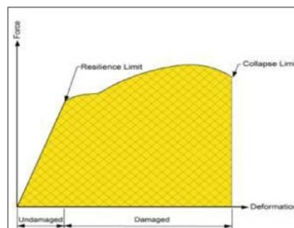
Figure 2. Toughness defined as area below force-deformation curve (yellow) (PIANC Report 137, 2014).
