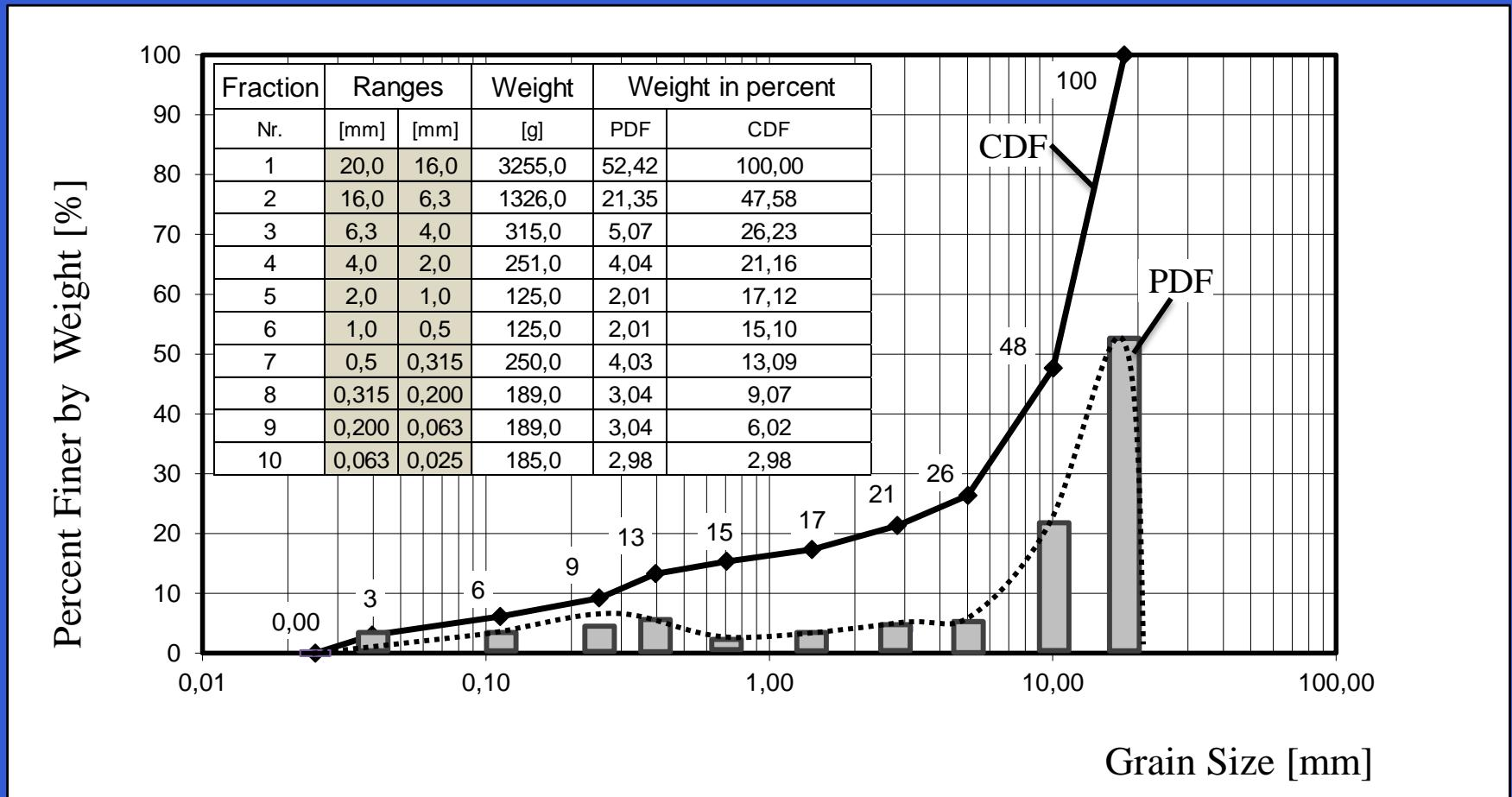
**Particle size distribution of investigated soil and Probability density function of its fractions ; CDF: Cumulative Distribution Function ~ PSD, PDF: Probability Distribution Function**
