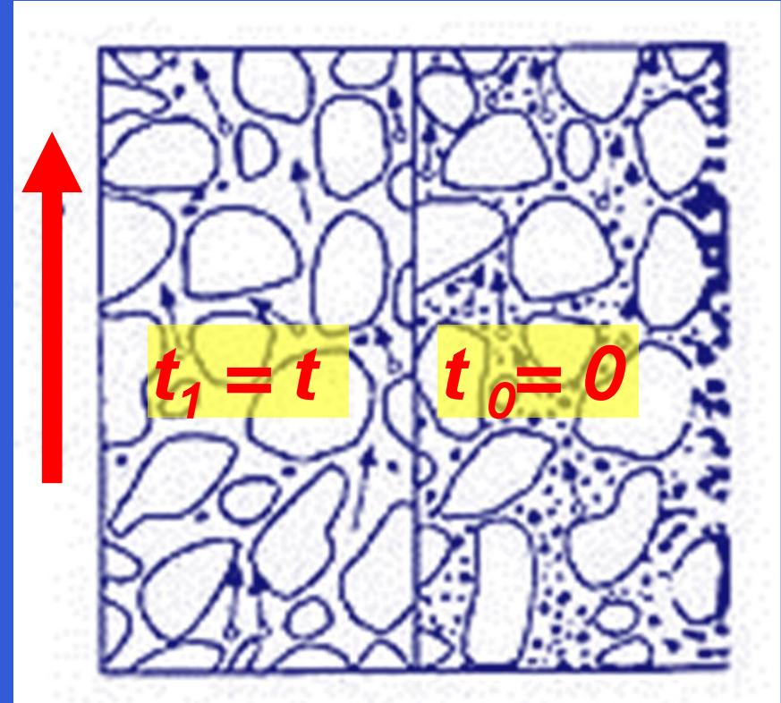
Left: a widely graded soil ; Right: the changes of the soil structure due to water flow
