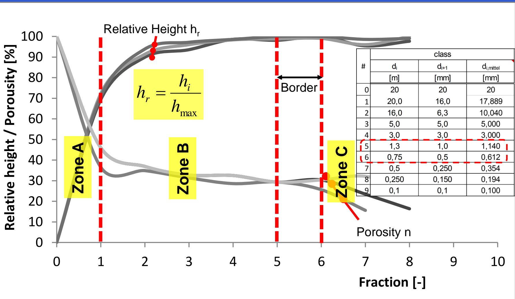
The results of three sequential fill tests (SFT) on the investigated soil
