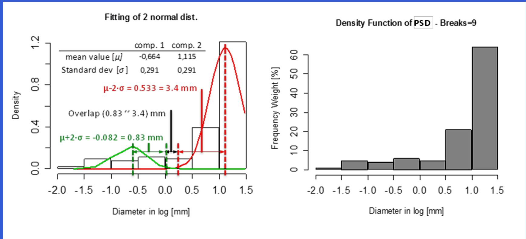
PDF of particle size distribution fitted with a parametric algorithm in R - Right: histogram of particles is clearly suggestive of a two-component mixture; Left: the fitted Gaussian components
