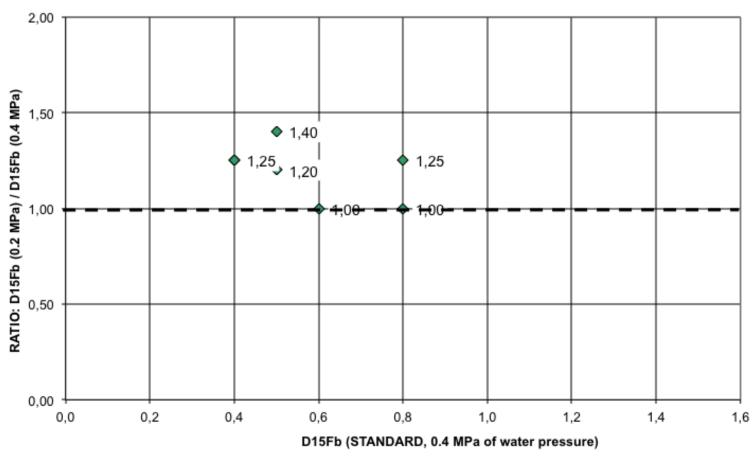
The hydraulic gradient represented in the NEF tests is many times higher than the expected in a real dam. For the design of new dams, we do recommend using the modern filter criteria, but if we are assessing an existing dam, we possibly had to use less restrictive criteria.
