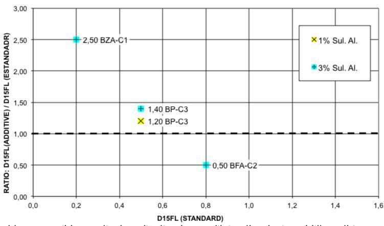
Apart from possible practical application for modifying the design of filters; this conclusion demonstrates that the dispersivity and, more certainly, the water chemistry and composition of the clay are variables that influence the design of granular filters.
