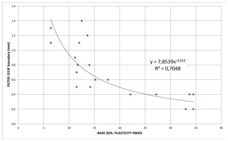
Base soil plasticity by itself has an important influence, BUT in our samples, a high base soil plasticity index also means a high base soil fines content. Therefore the base soil plasticity has influence in the boundary filter, but it is not as important as the PSD
