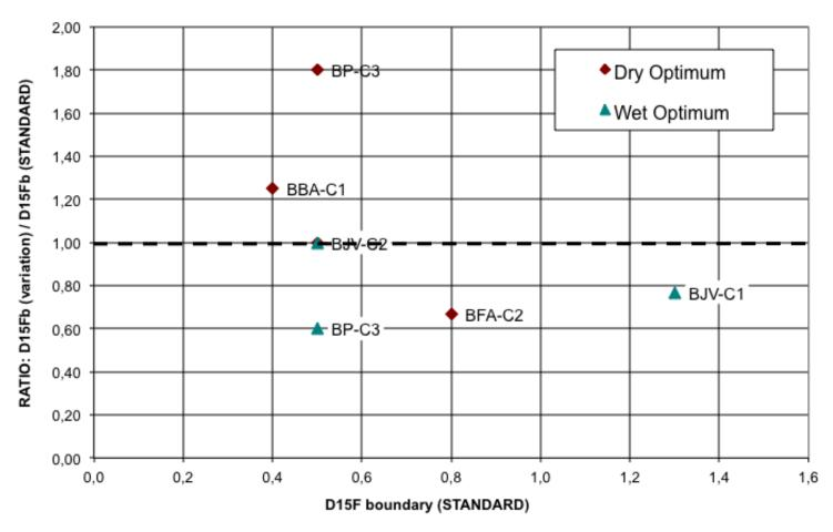
clay core should be compacted at the optimum water content. zones of higher moisture content and lower density than that expected during construction can be more susceptible to internal erosion.
