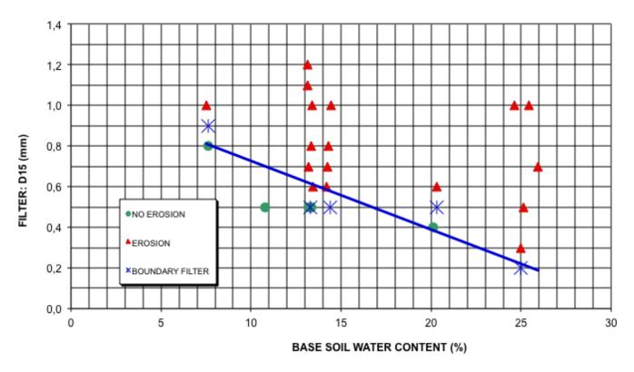
For BP-C3 base soil sample, the boundary filter D15F<sub>b</sub>, decreases as the base soil water content increases, with a variation from 0.9 mm to 0.2 mm. This result is quite surprising.
