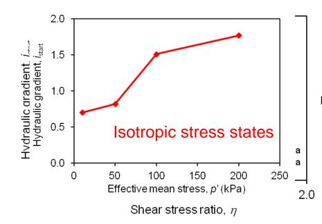
Under the same shear stress ratio,  $i_{\text{start}}$  increases with confining stress
