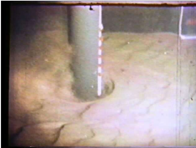
Unprotected pile (1978: Model tests by Zanke)
