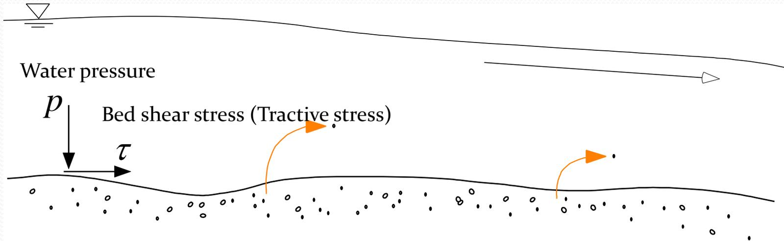
Erosion rate  $E$  = Volume of soils eroded from unit surface area during unit time
