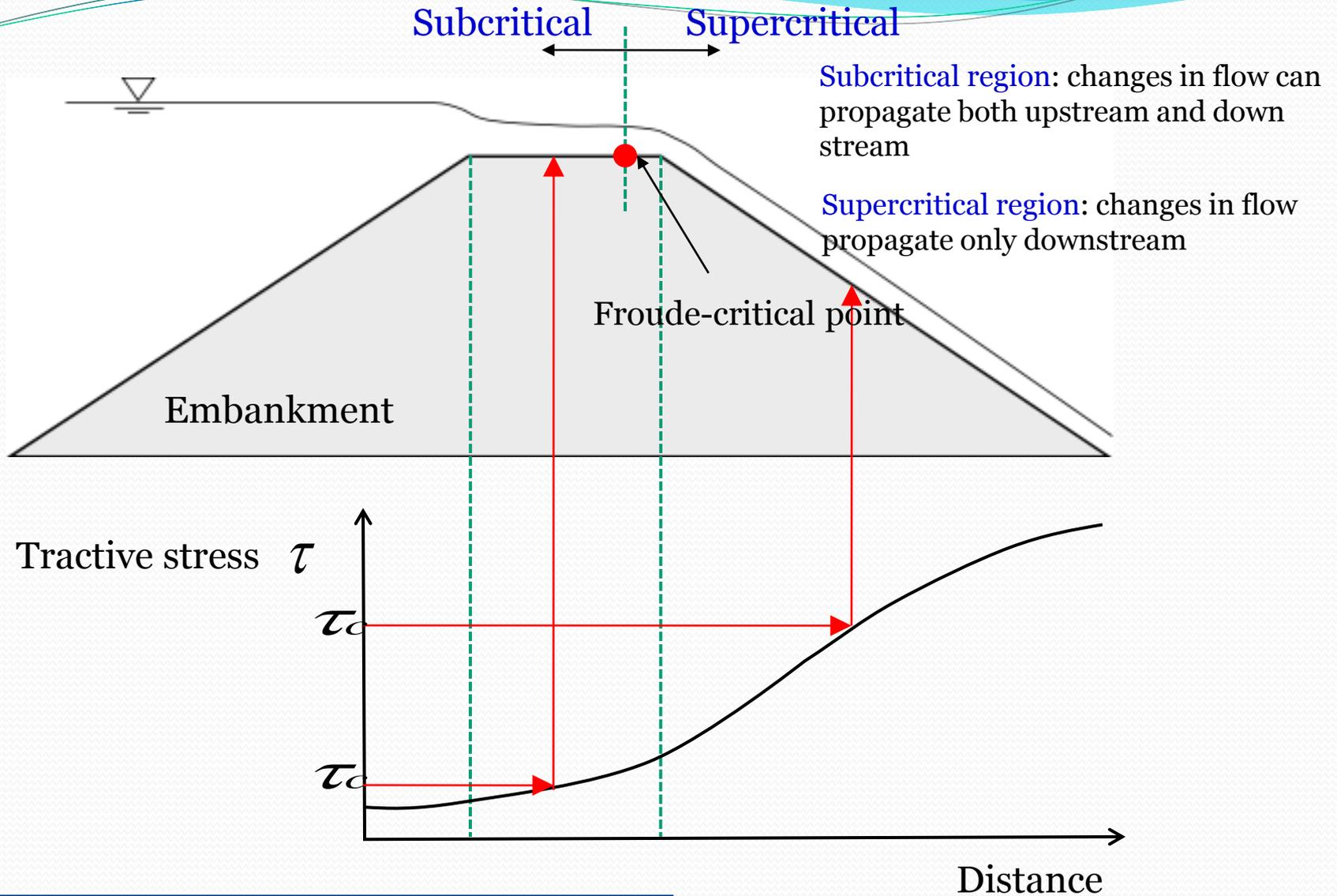
Where the friction stress reaches the critical stress and the erosion start
