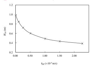
Right figure shows the relationship between  $k_{BF}$  and  $H_{PF}$ , it is found from the figure that the value of  $H_{PF}$  increases and converges in the vicinity of 1.0 m with decreasing  $k_{BF}$ . Lesspermeable backfill is also effective in increasing stability against boiling of the bottom soil.
