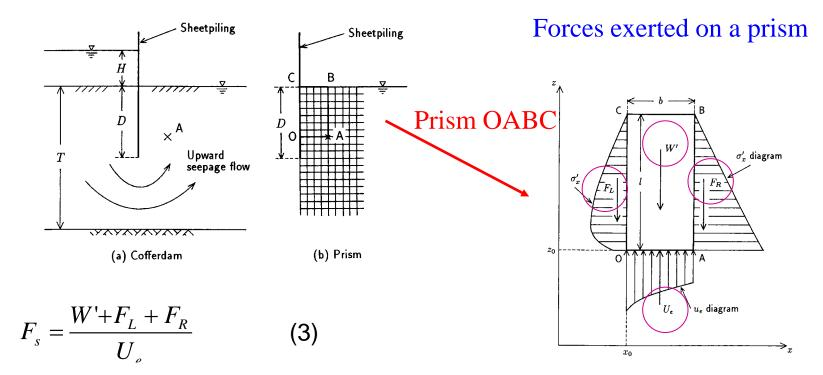
The critical prism is determined by the condition that the minimum safety factor  $F_{s \min}$  becomes just equal to 1.0 among all of the prisms.
