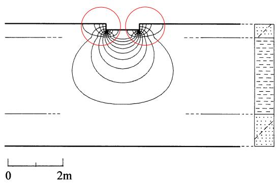
Flow net when not considering backfills
