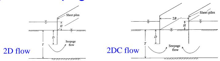
In the excavation of soil between double sheet pile walls, as shown in the right figure, seepage water concentrates into the soil two-dimensionally from the outside, which is called two-dimensional concentrated flow (2DC flow). The 2DC flow of water lowers the safety factor regarding the seepage failure than 2D flow.
