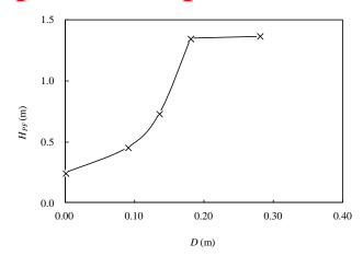
Right figure shows the relationship between the depth of the panel D and the theoretical critical hydraulic head difference  $H_{PF}$ .
