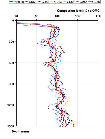
Compaction level recalculated from volumic weight measurements (gamma probe)
