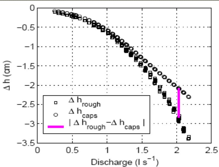
*Head loss for increasing flow discharge with plexiglass caps (circle) and with sediment cores (square): excess of bed shear stress due to mud roughness for a given discharge is proportional to the distance between the two curves as displayed by the thick vertical line.*
