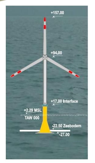
The GBF is a concrete cylindrical/conical structure, held in place by its own gravity.
