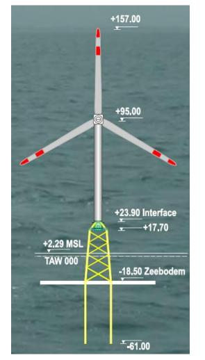
The jacket foundation is a steel structure with four legs connected to each other with braces.
