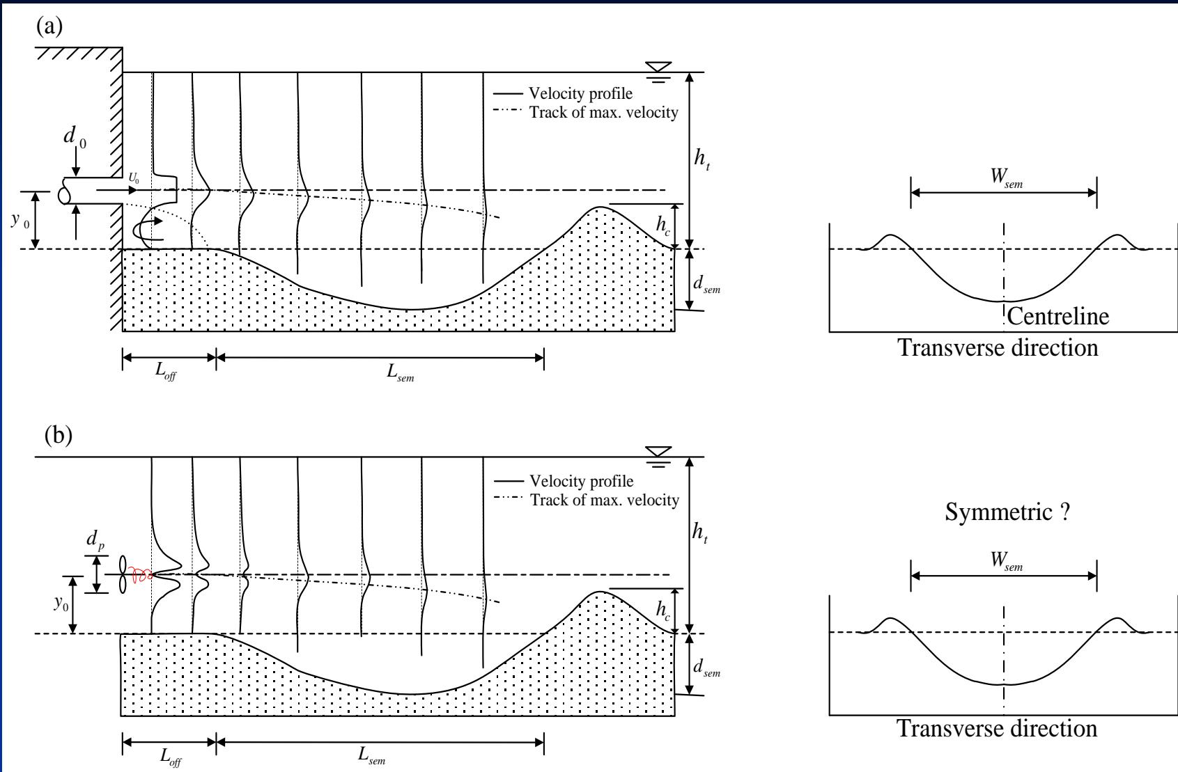
Scour by (a) offset jet; and (b) propeller jet
