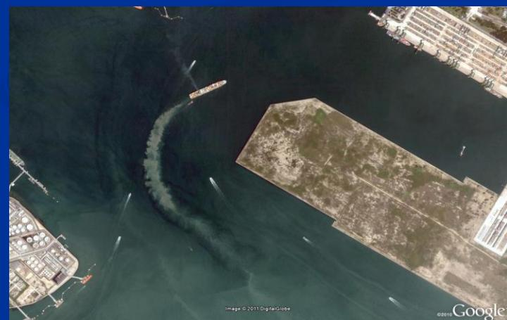
Propeller wash induced erosion
