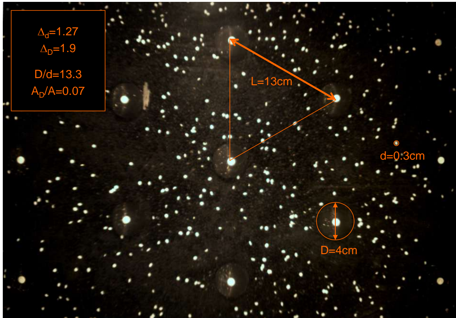
Figure 6. Path of macro-roughness elements in RBLD configuration.
