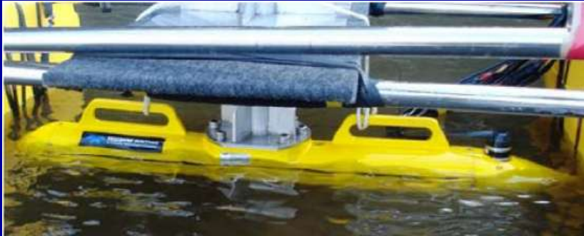
Fig.04 Multi-angle swath bathymetry system (C3D, Teledyne BENTHOS) mounted on broadside of boat
