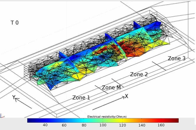
A set of electrical measurements was acquired before the beginning of the infiltration
