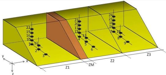
24 moisture probes were installed into the dike to monitor the evolution of the infiltration.
