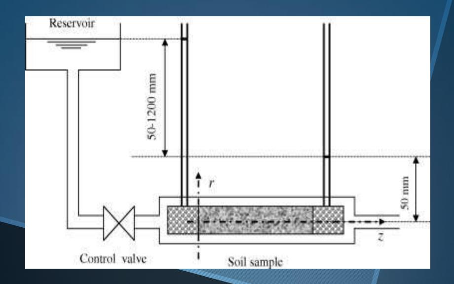
Schematic diagram of the hole erosion test
