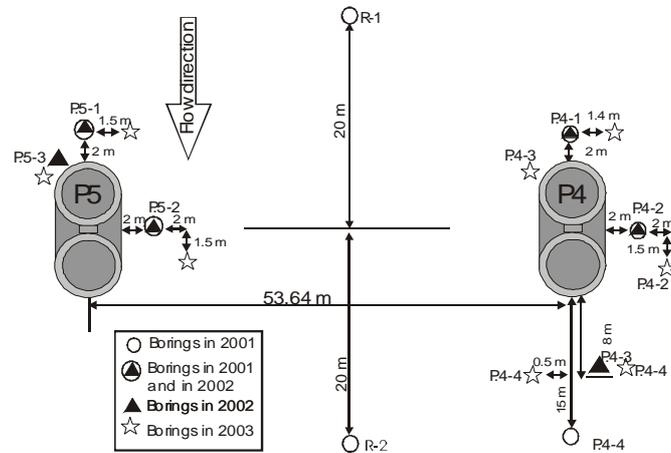
Figure 2. Borings around piers 4 (P4) and (P5).
