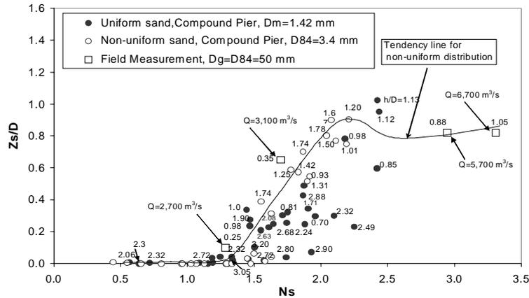
Figure 6.  $Z_s/D$  vs  $N_s$  for compound piers.
