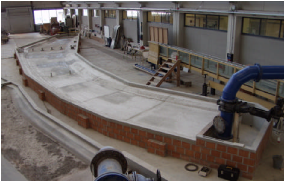
Figure 1: Physical model of the Salzach river section
