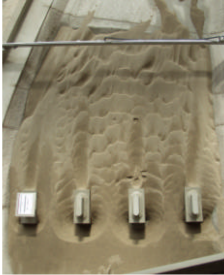
Figure 2: Variant A – Local erosion of the bed
