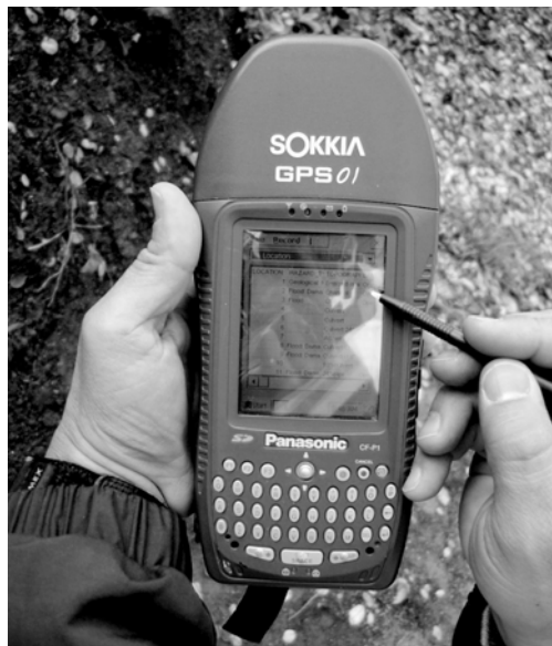
Figure 3. Jetstream equipped PDA for consistent field data gathering.
