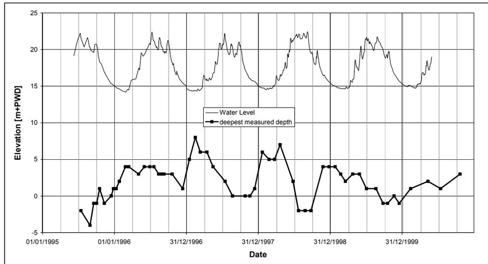
Figure 3. Development of river depth along the bend.
