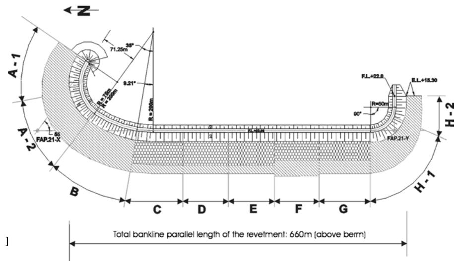
Figure 6. Plan view of Bahadurabad test revetment. (FAP 21, 2001)
