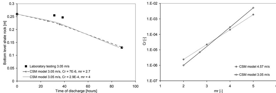
Figure 6. a) Comparison of computed and laboratory measured scour; b)  $C_r$ - $m_r$  relationships as calibrated.
