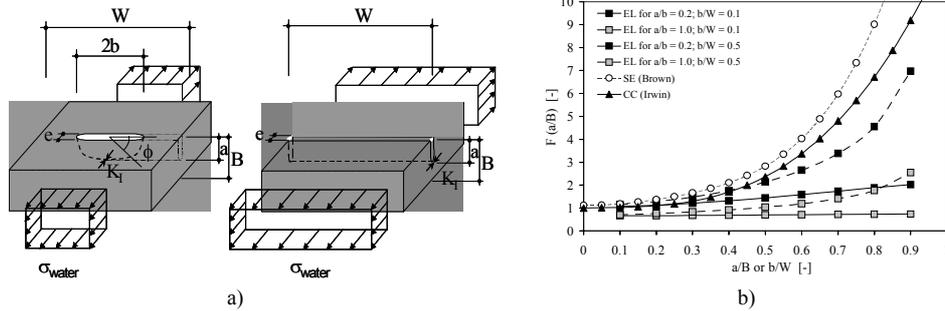
Figure 2. a) Main configurations for partially jointed media; b) Boundary correction factor F.
