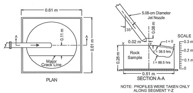
Figure 5. Plan and side view of test installation at IIHR (Iowa) on shale-rock samples (Nakato, 2002)
