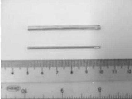
Figure 6. Pins used for the model tests.
