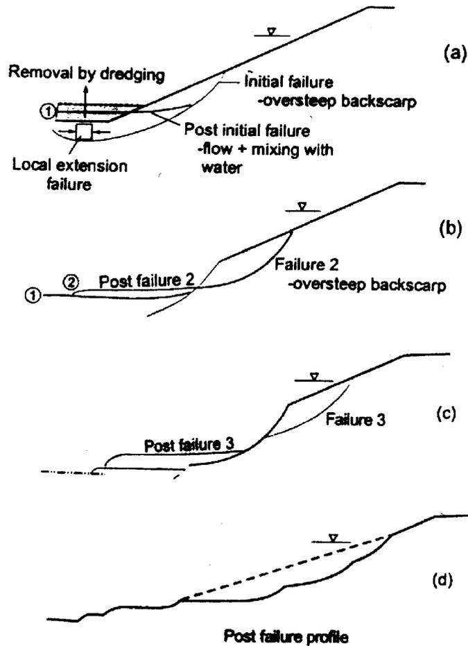
Figure 2 Retrogressive flow failure due to dredging (after Hight et al. 1999)
