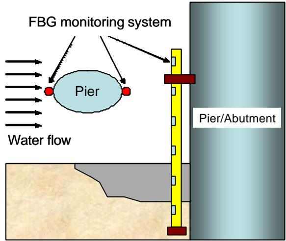
Fig. 2 The FBG scour monitoring system --Model II
