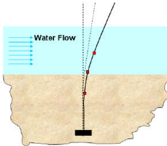
Fig. 1 The FBG scour monitoring system --Model I
