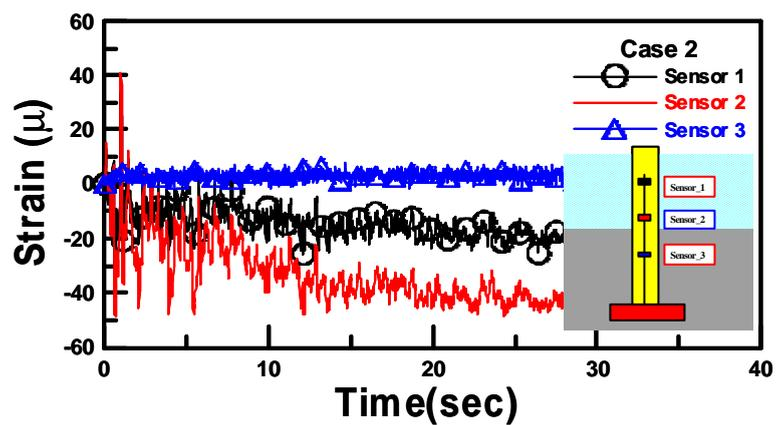
Fig. 4 Model I- sensor\_2 emerges out the sediment
