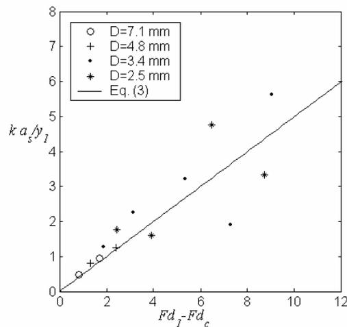
Figure 4. The product between the pressure correction coefficient  $k$  and the dimensionless maximum scour  $a_s/y_1$  as a function of  $Fd_1 - Fd_c$ .
