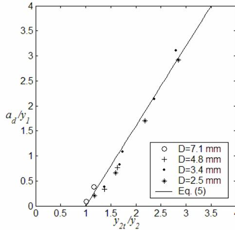
Figure 7. The ratio between measured deposit height  $a_d$  and upstream flow depth  $y_1$  as a function of  $y_{2t}/y_2$ .
