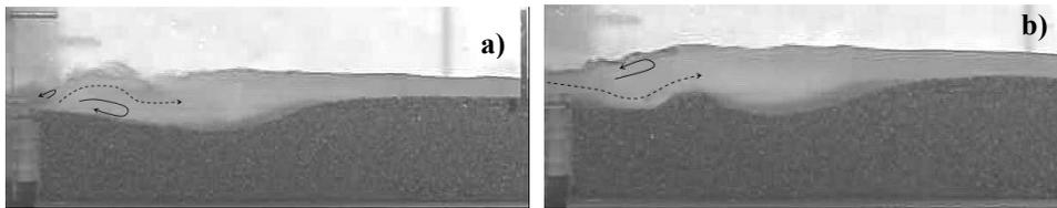
Figure 3. Side view of the free surface and bed profile configuration type I (a) and II (b). Continuous arrows indicate the pattern of macro-vortex system, dashed lines the direction of main flow.
