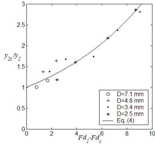
Figure 6. The ratio between theoretical flow depth  $y_{2t}$ , in the case of fixed bed condition and the measured flow depth  $y_2$  as a function of  $Fd_1 - Fd_c$ .
