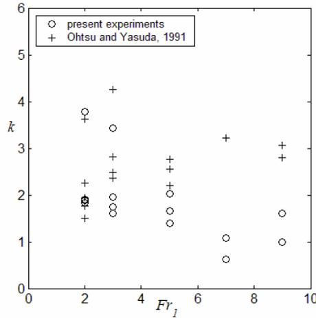
Figure 5. The pressure correction coefficient  $k$  as a function of the Froude number of the flow at the upstream boundary  $Fr_1$ .
