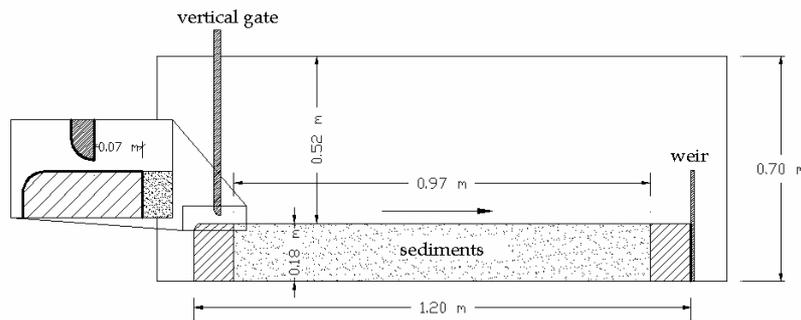
Figure 2. Experimental equipment (the arrow indicates the direction of main flow).
