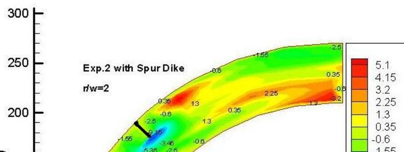
Figure 2. Scour pattern around spur dike for  $Q = 20(\text{L/s})$  and  $Fr = 0.4$  with  $R/W=2$
