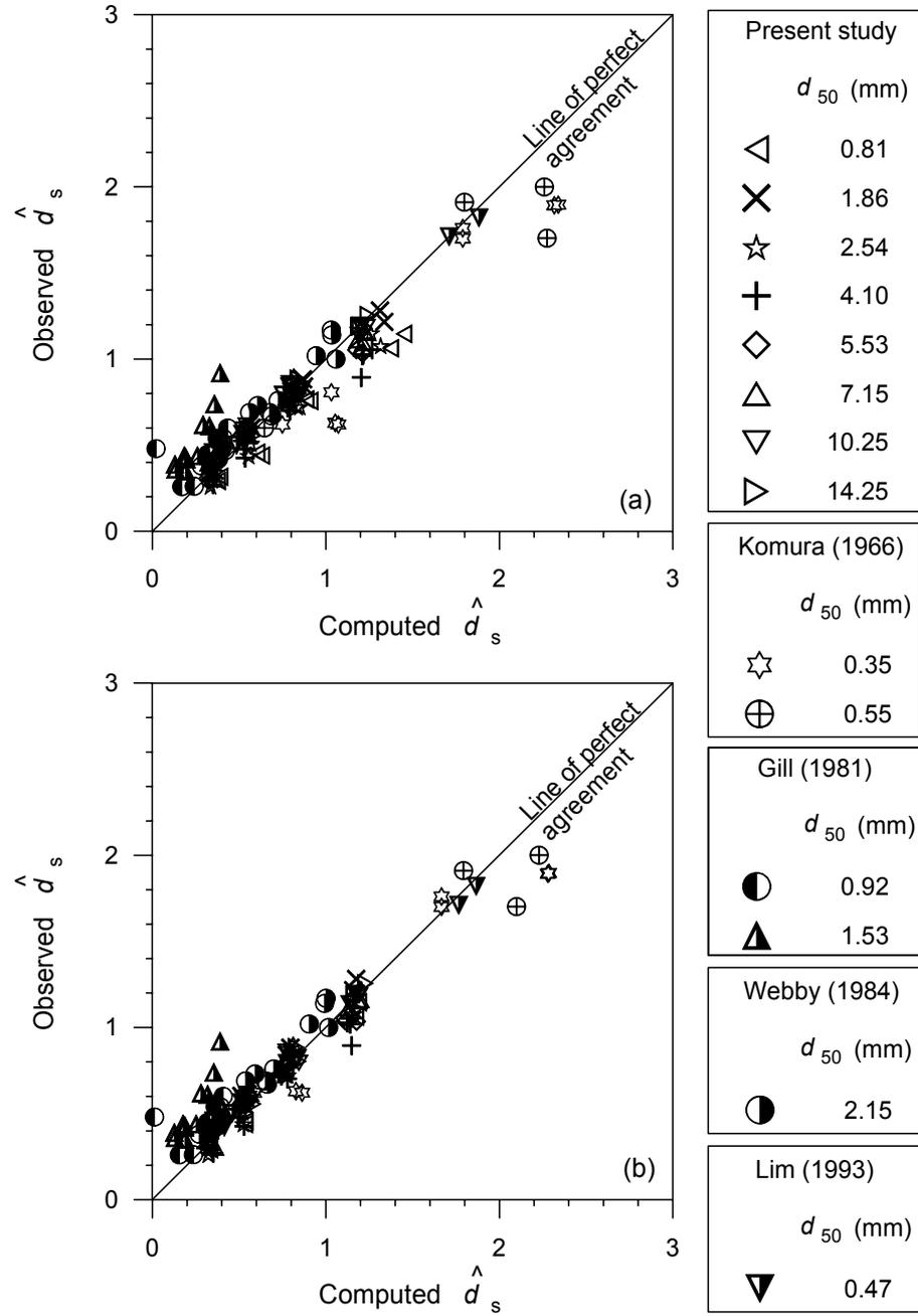
Figure 2. Comparison between the experimental data and computed values of equilibrium scour depths  $\hat{d}_s$  using clear-water scour model (a) with sidewall correction and (b) without sidewall correction.
