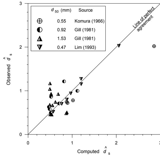
Figure 3. Comparison between the equilibrium scour depths  $\hat{d}_s$  computed using live-bed scour model and the experimental data.
