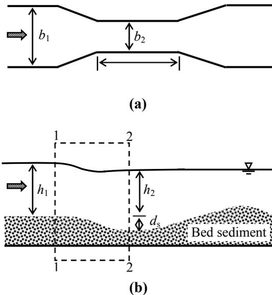
Figure 1. Schematic view of a channel contraction at equilibrium scour condition: (a) top view and (b) side view.
