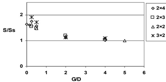
Figure 3. Equilibrium scour-hole depth plotted against pier spacing
