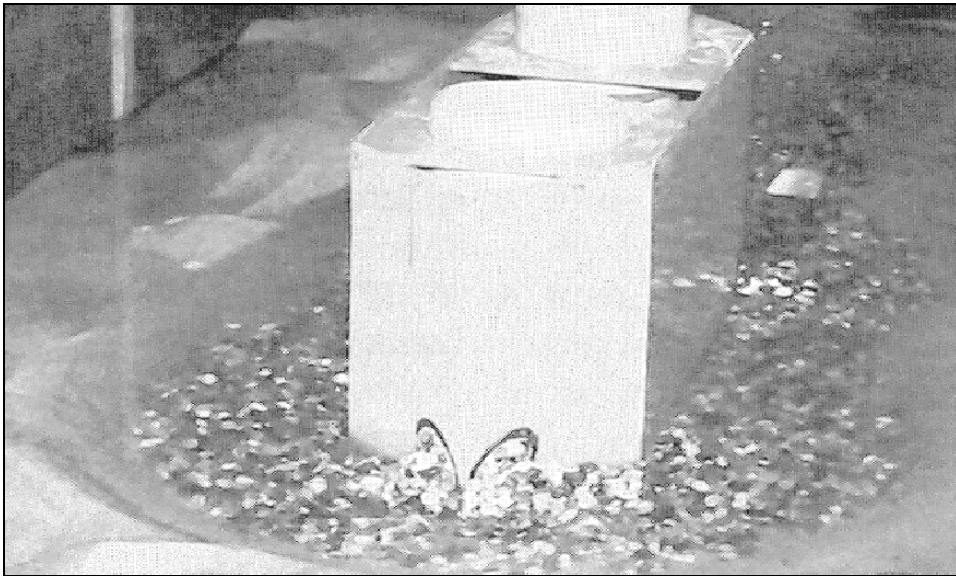
Figure 1. Laboratory test of a hollow pier filled with rip-rap (source: Zanke, 1994).
