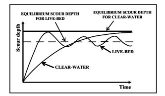
Figure 1. Scouring in clear-water and live-bed conditions (Raudkivi, 1998).
