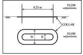
Figure 6. Position of collar around a rectangular pier.
