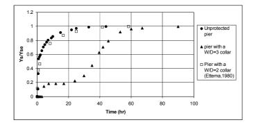
Figure 4. Time development of scouring with collars of different sizes.
