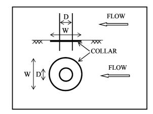
Figure 2. Position of collar around a circular pier.
