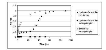
Figure7. Comparison of scouring rate at a rectangular and a circular pier.
