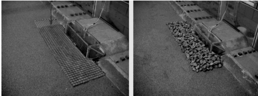
Figure 2. Experimental set-up of a 0.3-m-wide apron placed around the abutment. Left; CTB apron placed on the surface. Right; riprap apron placed on top of the average bed level.
