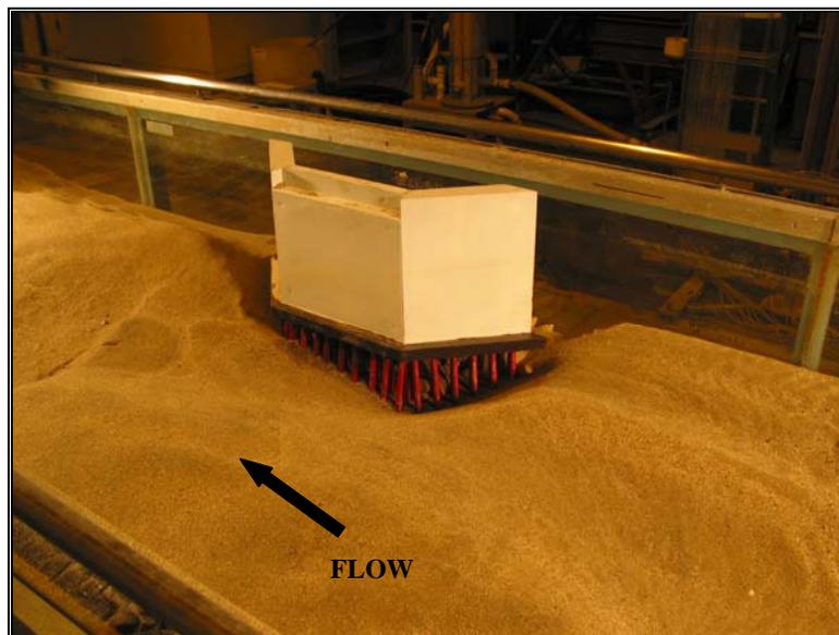
Figure 3. Scour development when only the erodible embankment was armored.
