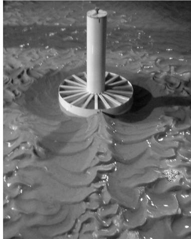
Figure 3 Result of scour test with current (Test 2)
