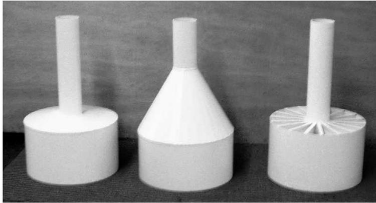
Figure 1 Foundation models used in testing – L-R: concrete-conical-girder
