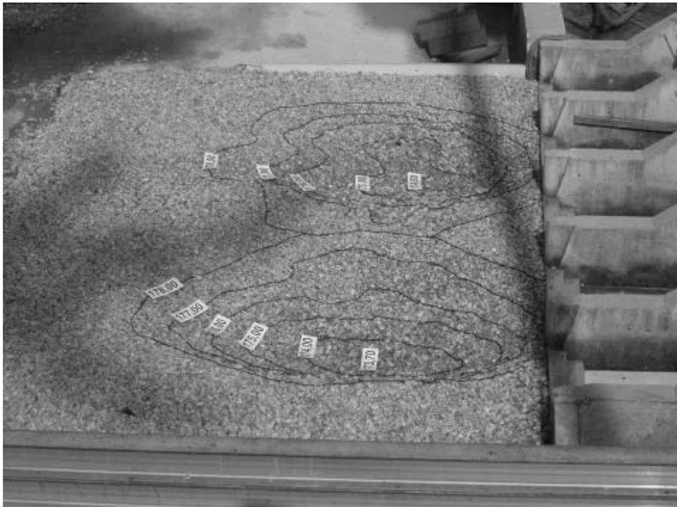
Figure 1: River bed mapping with wool threads
