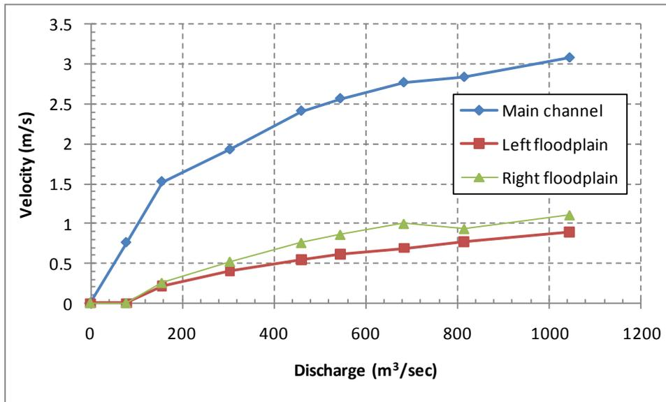
**Figure 44 – Relationship between Discharge and Velocity.**
