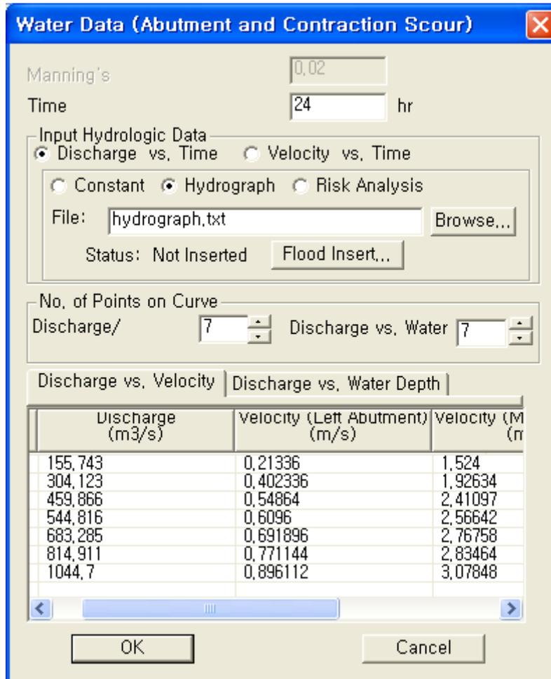
Figure 43 – Water data input window for abutment and contraction scour.
