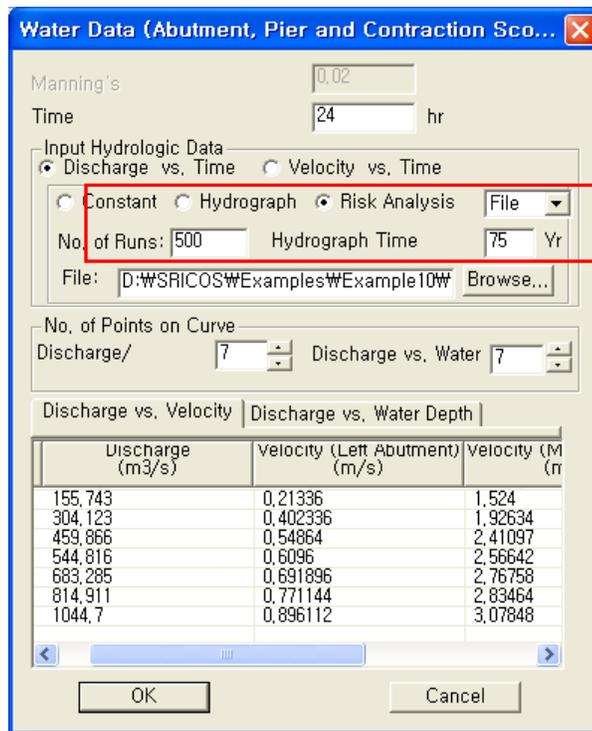
Figure 54 – Water Data input window for Risk Analysis using existing hydrograph.
