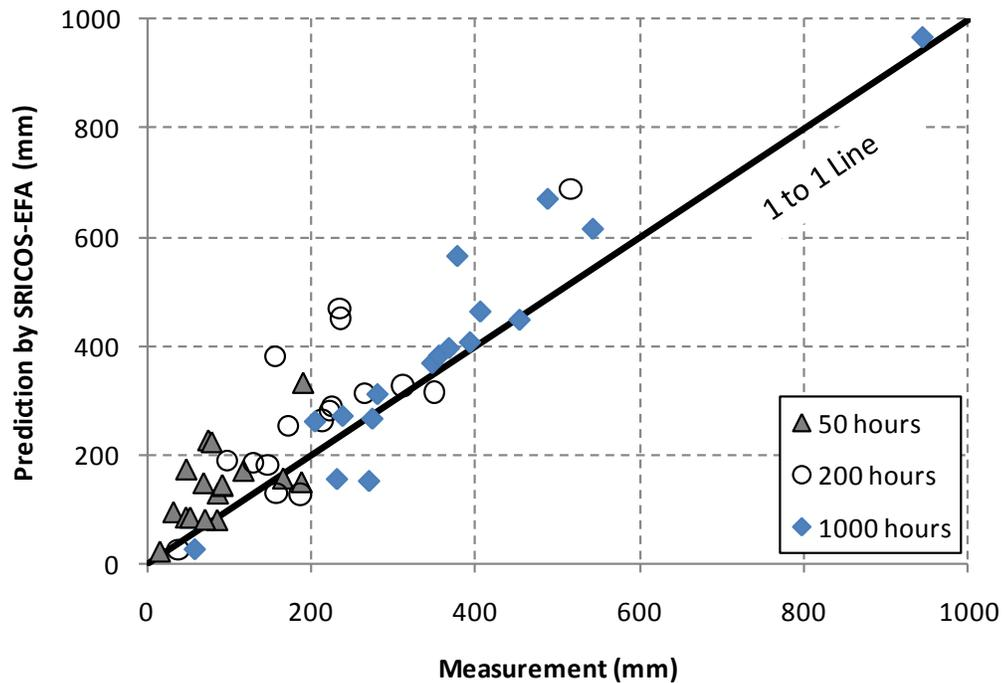
**Figure 24 – Comparison of abutment scour depth in Porcelain clay between prediction by SRICOS-EFA and measurement.**
