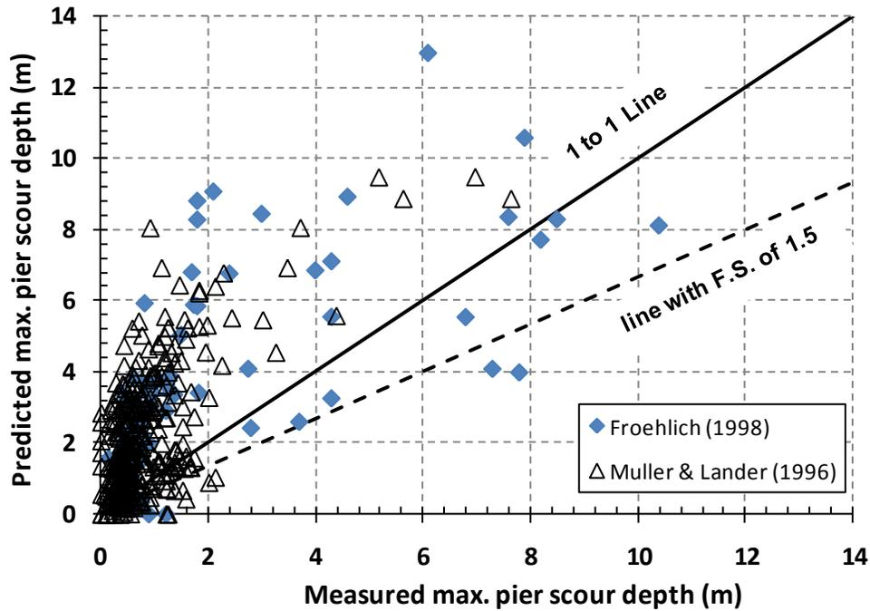
**Figure 15 – Predicted maximum scour depth versus databases from Froehlich (1998) and Muller and Lander (1996).**
