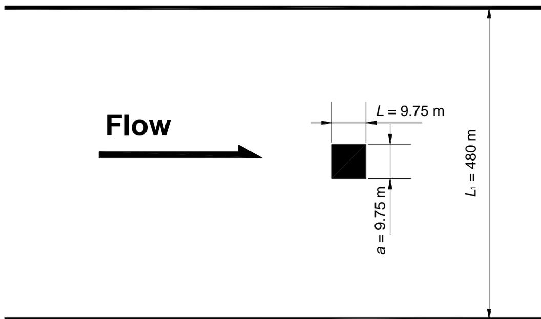
Figure EX. 6 – Channel and pier geometry.
