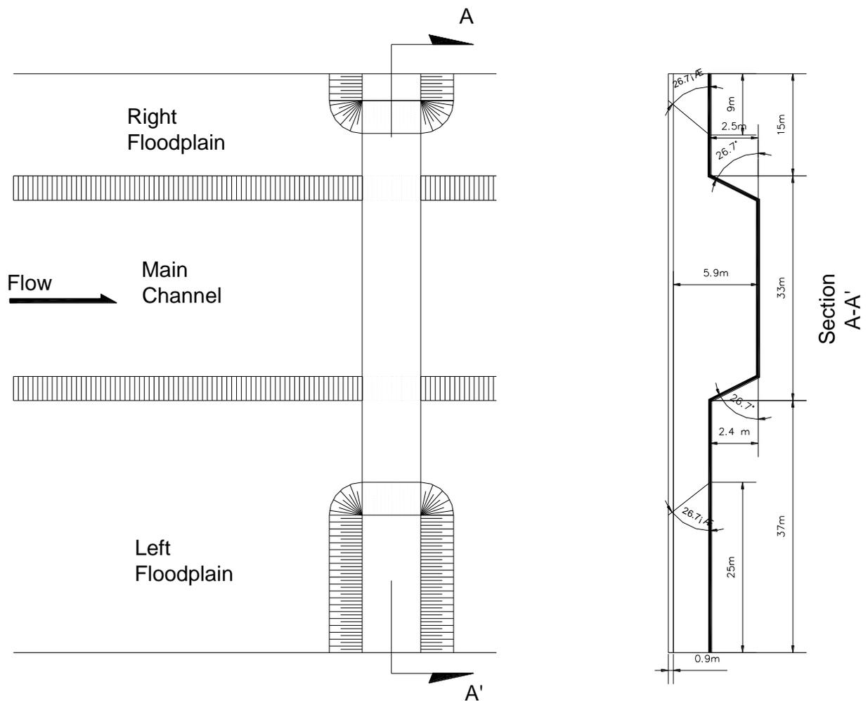
Figure EX. 12 – Channel geometry (Example 4).
