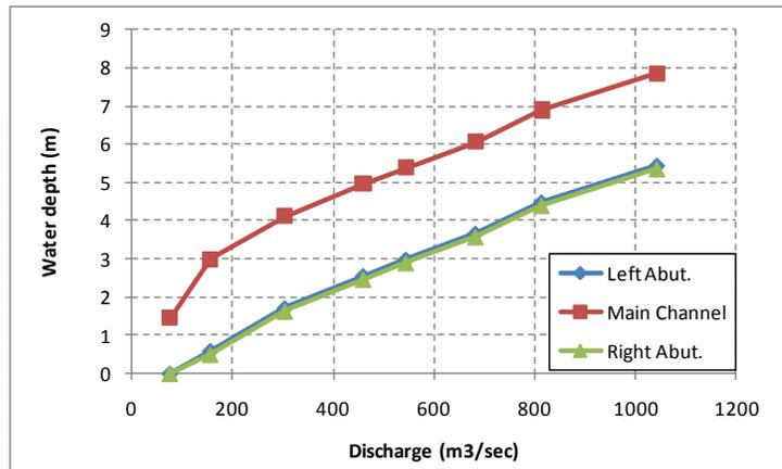
**Figure EX. 16 – Relationship of Discharge vs. Water depth (by HEC-RAS run).**
