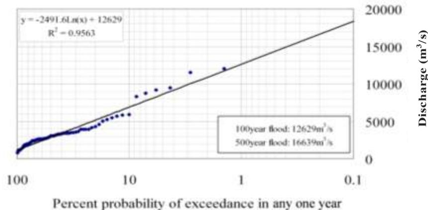
**Figure 14 – Flood frequency curve obtained from measured discharge hydrograph. (Briaud *et al.*, 2003)**
