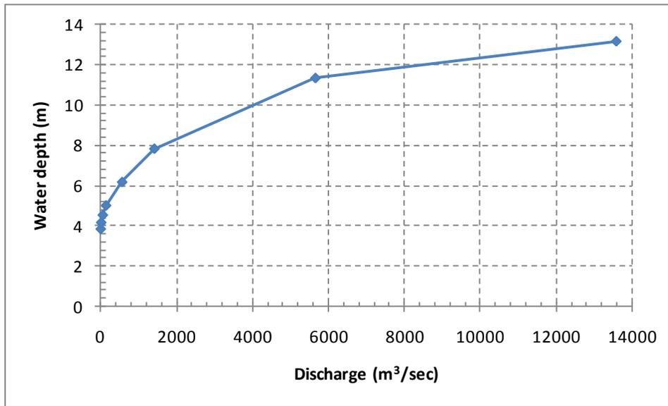
**Figure 35 – Relationship between Discharge versus Water depth from HEC-RAS results.**
