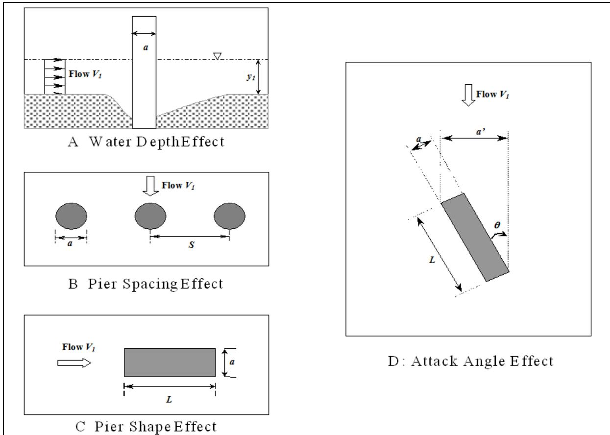
**Figure 9 – Schematic definition of pier parameters.**
