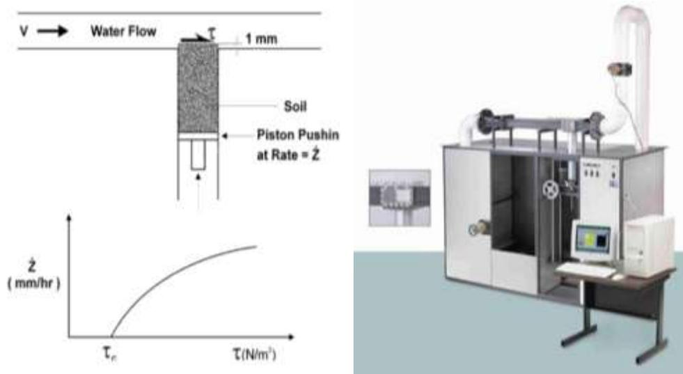
**Figure 1 – EFA (Erosion Function Apparatus) to measure erodibility (Briaud *et al.*, 1999).**
