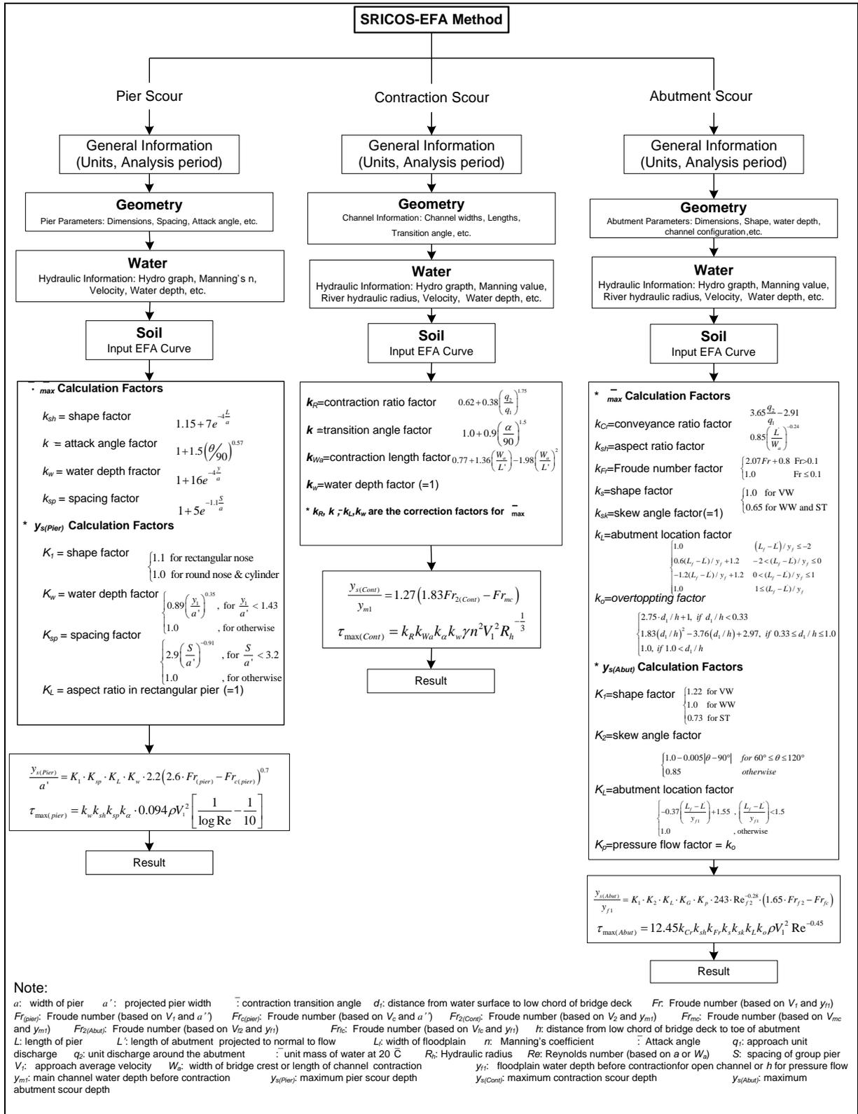
**Figure 25 – Procedure of SRICOS-EFA method.**
