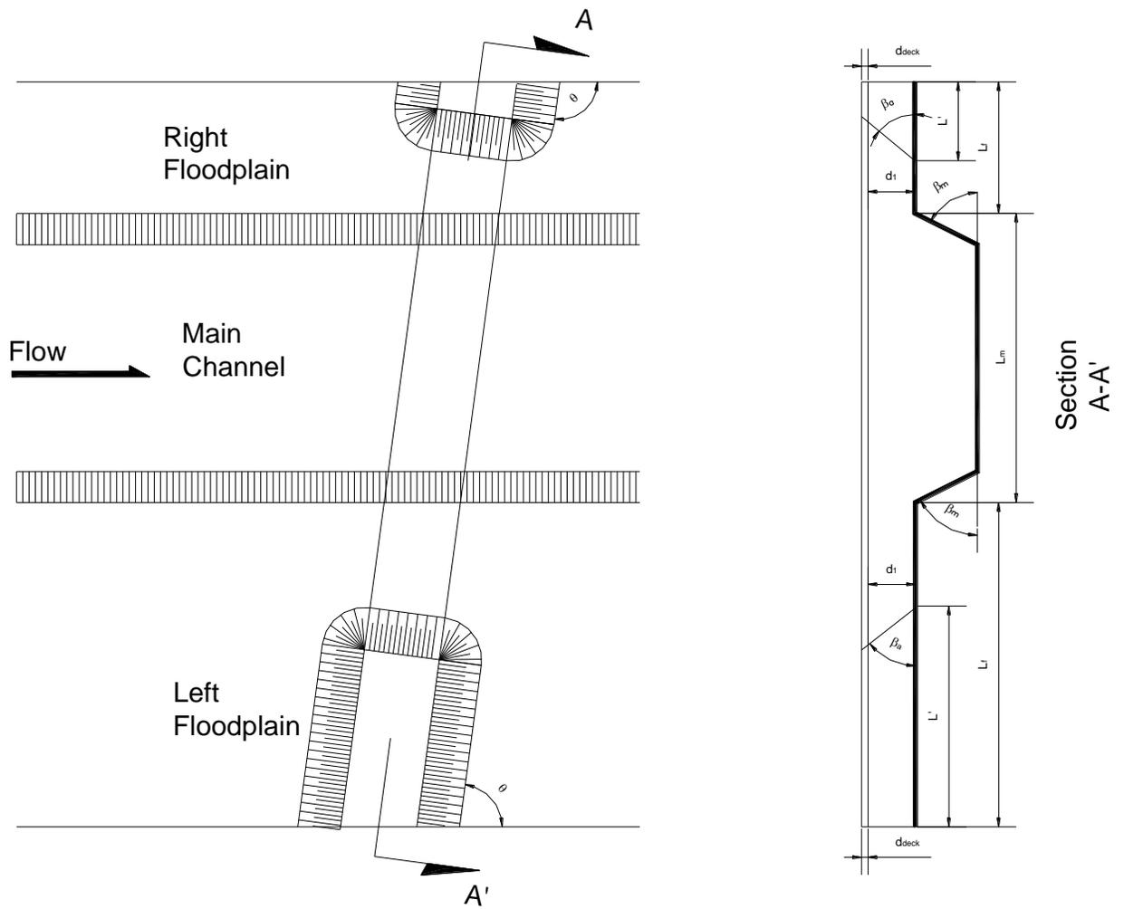
Figure 12 – Schematic definition of abutment scour parameters.
