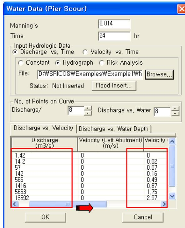
Figure 33 – Water data input window for pier scour.
