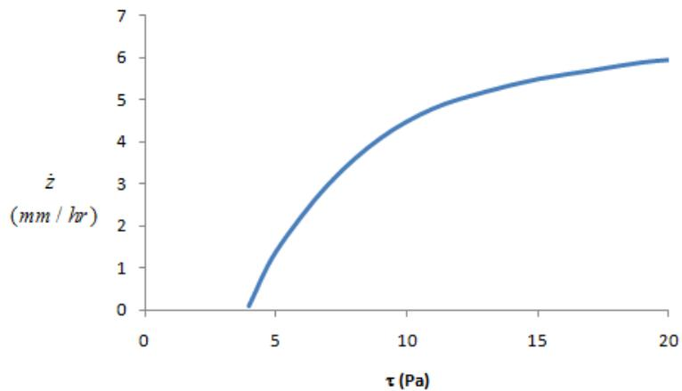
Figure EX. 2 – Erosion function of soil.
