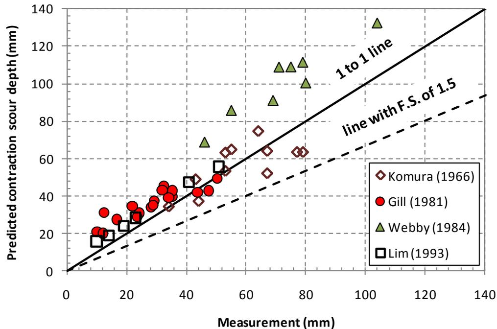
**Figure 16 – Predicted uniform contraction scour depths vs. measured uniform contraction scour depths in previous researches.**
