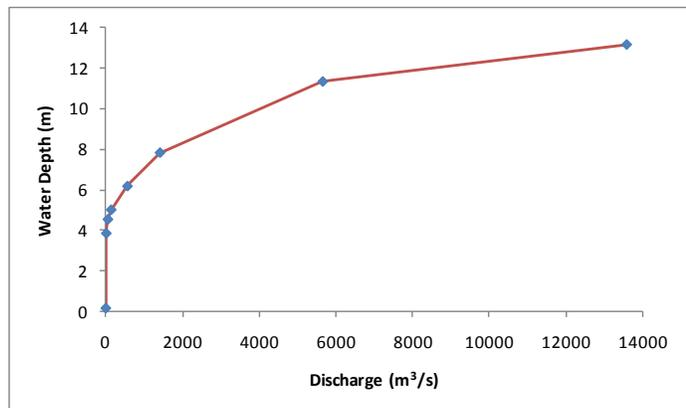
**Figure EX. 10 – Relationship of Discharge vs. Water depth (by HEC-RAS run).**
