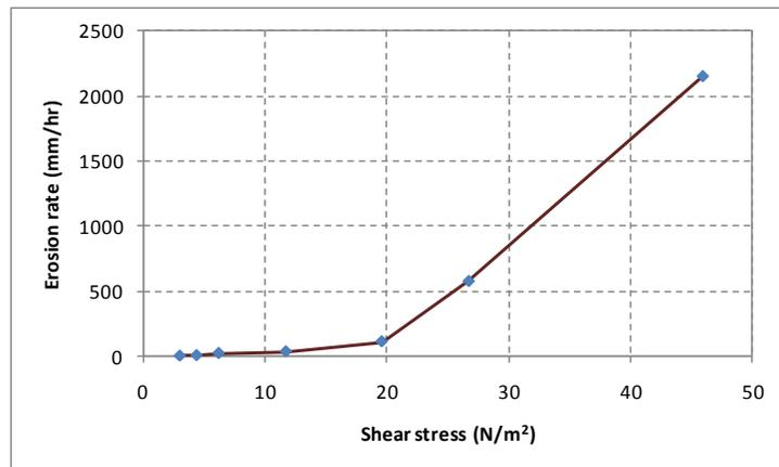
**Figure EX. 14 – EFA results for soil layer (Example 4).**
