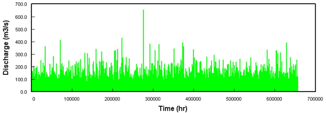
**Figure EX. 13 – Hydrograph from 1932 to 2006 (657,000 hours).**
