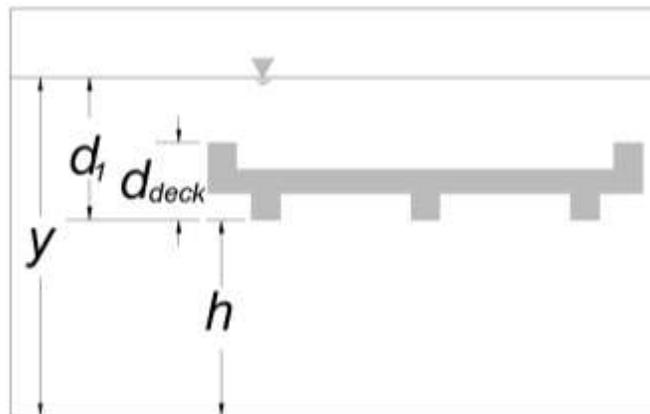
Figure 13 – Definitions for pressure flow near a bridge abutment.
