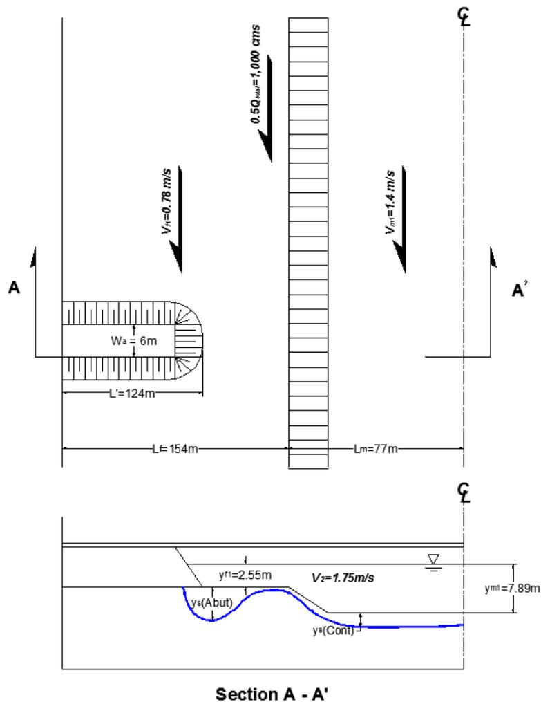
**Figure EX. 4 – Channel geometry.**
