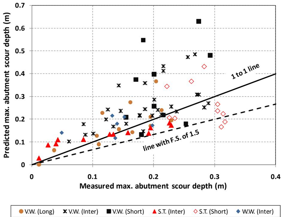
Figure 18 – Predicted maximum abutment scour depths vs. measured abutment scour depths in Sturm (2004).
