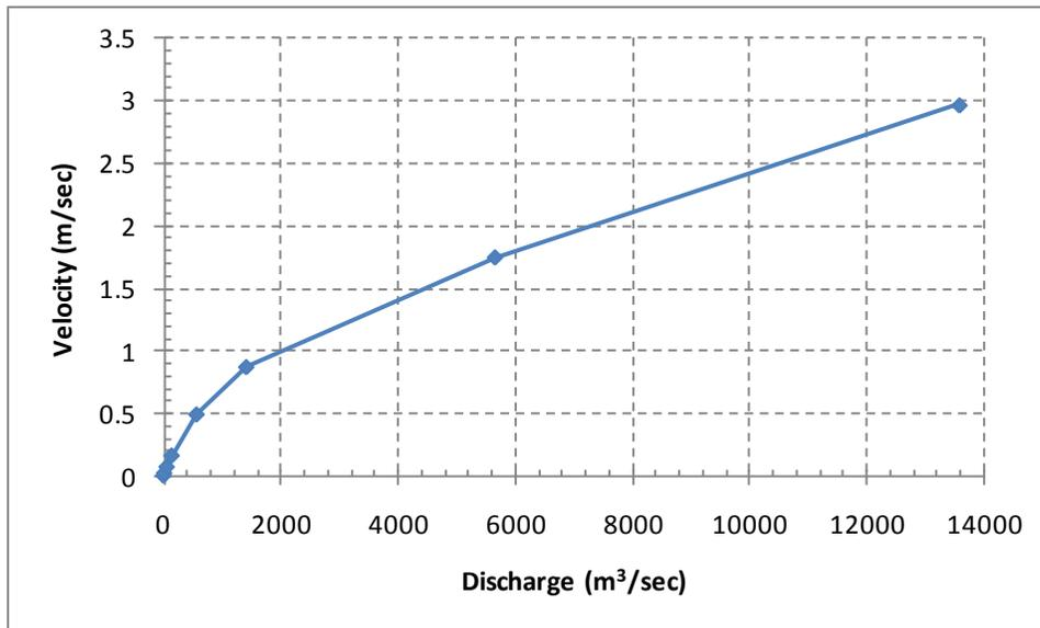
**Figure 34 – Relationship between Discharge versus Velocity from HEC-RAS results.**
