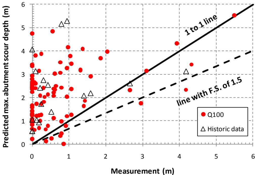
**Figure 20 – Predicted maximum abutment scour depths vs. measured abutment scour depths in Benedict and Caldwell (2006).**
