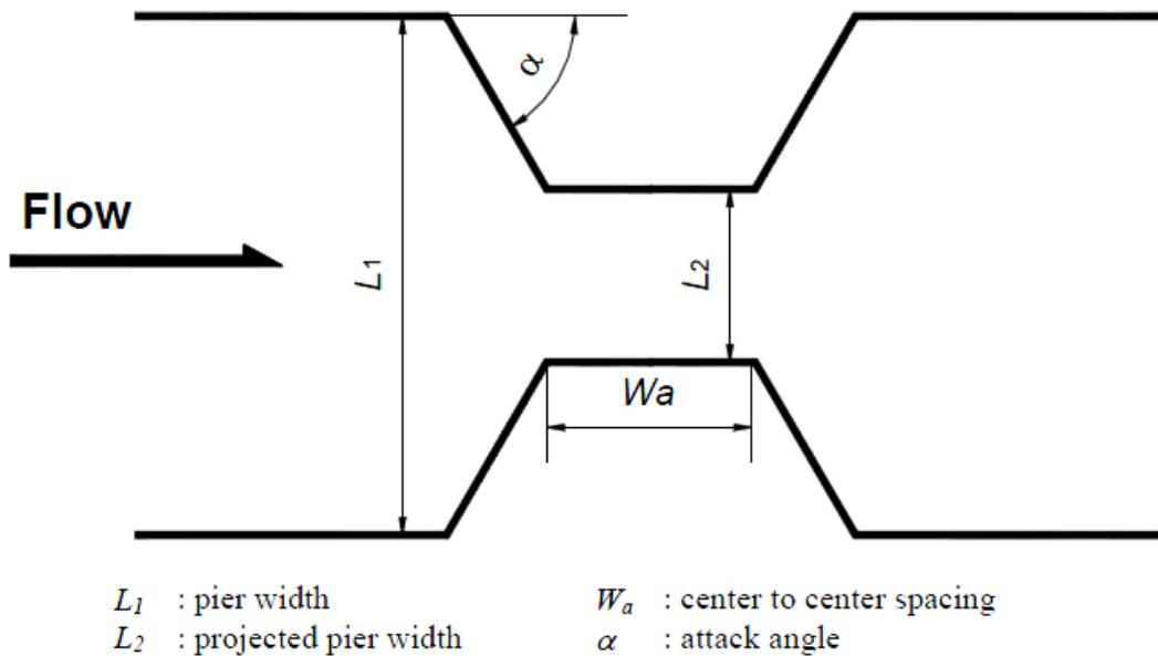
**Figure 38 – Schematics of contraction scour parameters.**
