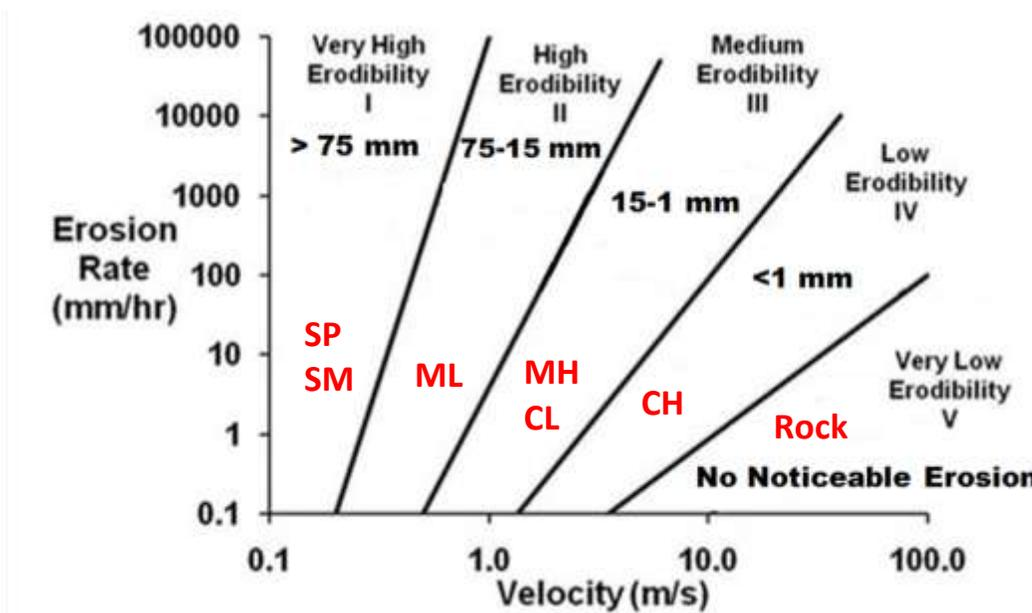
Figure 6 – PET erosion depth ranges shown on EFA categories.
