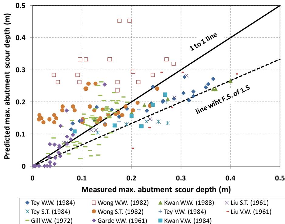
**Figure 17 – Predicted maximum abutment scour depth vs. measured maximum abutment scour depth in Froehlich (1989).**
