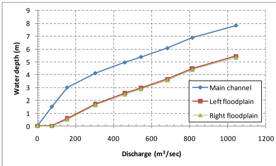
**Figure 45 – Relationship between Discharge and Water depth.**
