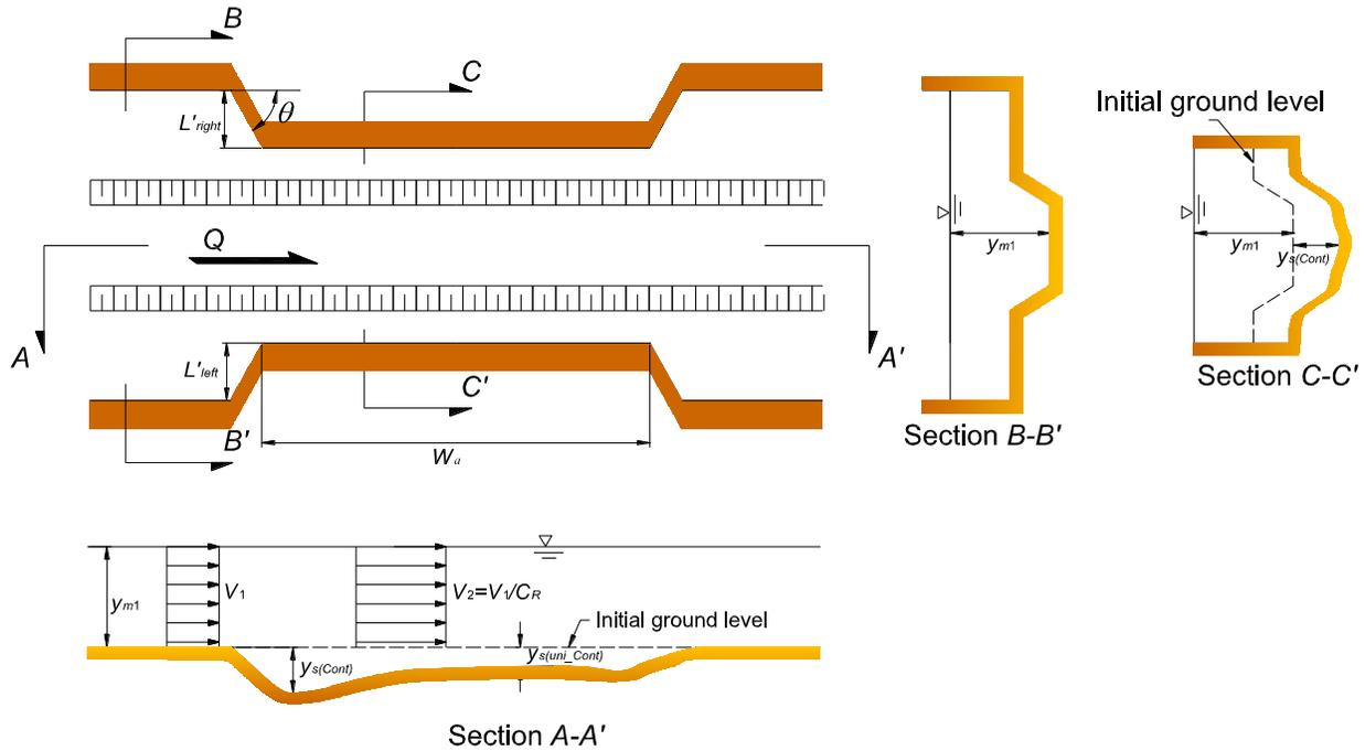
**Figure 10 - Schematic definition of contraction scour parameters.**
