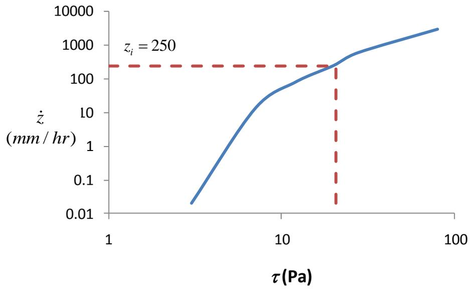
**Figure EX. 19 – Erosion function and initial erosion rate corresponding to the maximum velocity (Example 6).**
