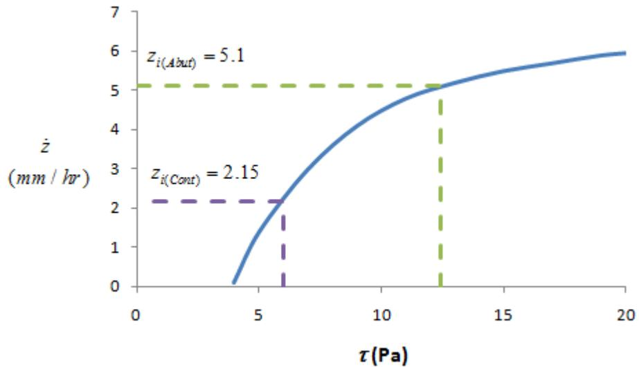
**Figure EX. 5 – Erosion function and initial erosion rate for contraction scour and abutment scour.**
