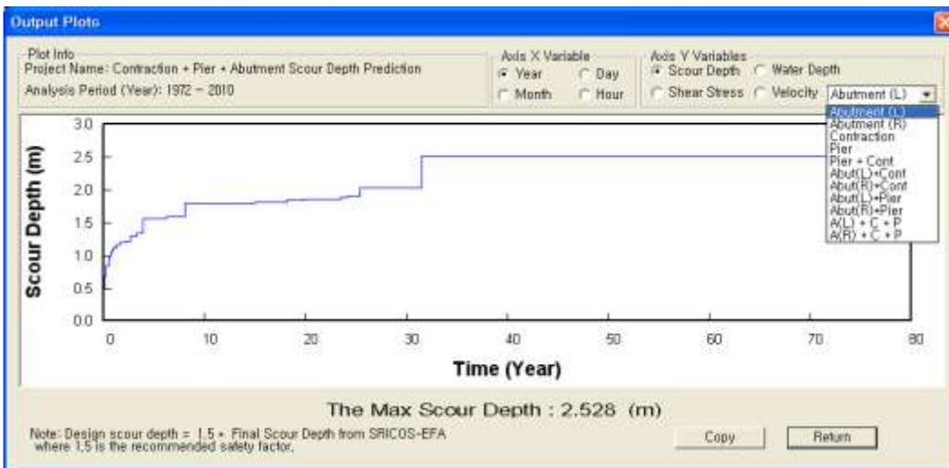
Figure 53 – Example of Output Plots (Scour Depth around the toe of Left Abutment vs. Time).
