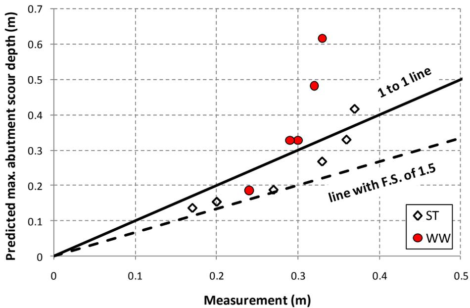
Figure 19 – Predicted maximum abutment scour depths vs. measured abutment scour depths in Ettema et al. (2008).
