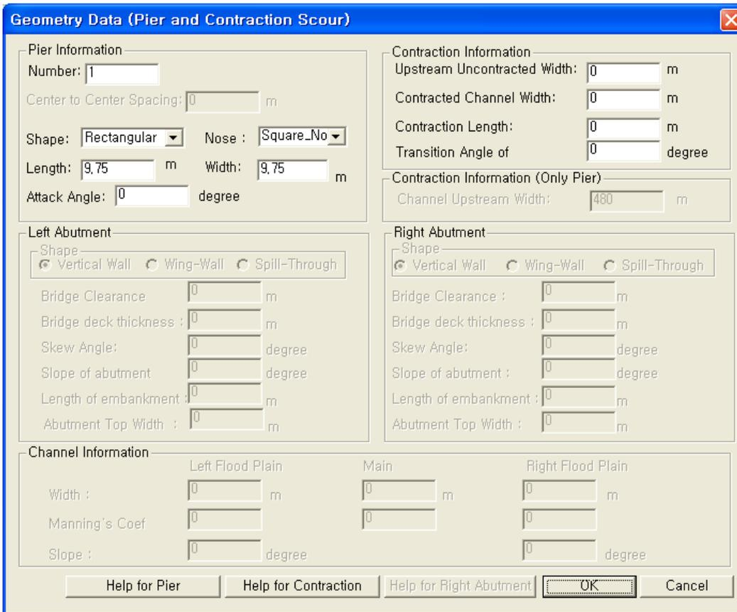
**Figure 39 – Geometry data input window for pier + contraction scour.**
