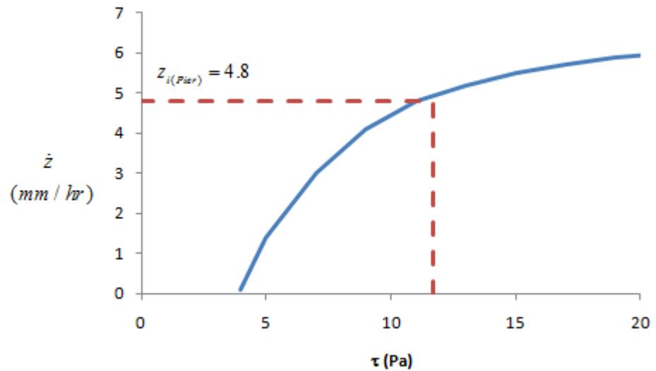
**Figure EX. 3 – Erosion function and the initial erosion rate of pier.**
