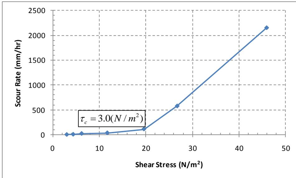
**Figure 32 – Typical EFA test result.**
