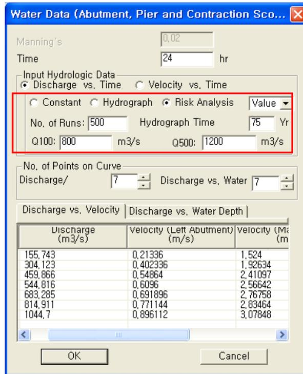
**Figure 59 – Water Data input window for Risk Analysis using Q<sub>100</sub> and Q<sub>500</sub> method.**
