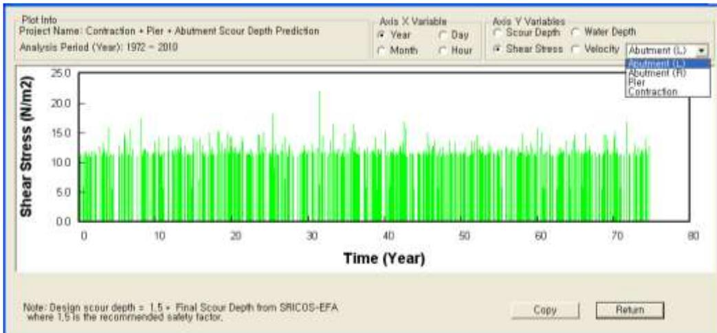
Figure 52 – Example of Output Plots (Shear Stress around the toe of Left Abutment vs. Time).
