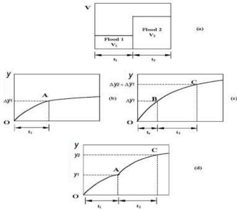
**Figure 7 – Scour due to a sequence of two flood events.**
