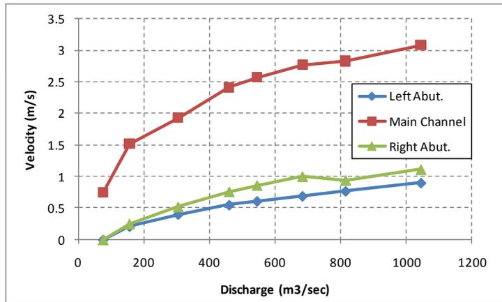
**Figure EX. 15 – Relationship of Discharge vs. Velocity (by HEC-RAS run).**
