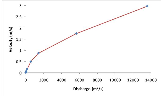
**Figure EX. 9 – Relationship Discharge vs. Velocity (by HEC-RAS run).**
