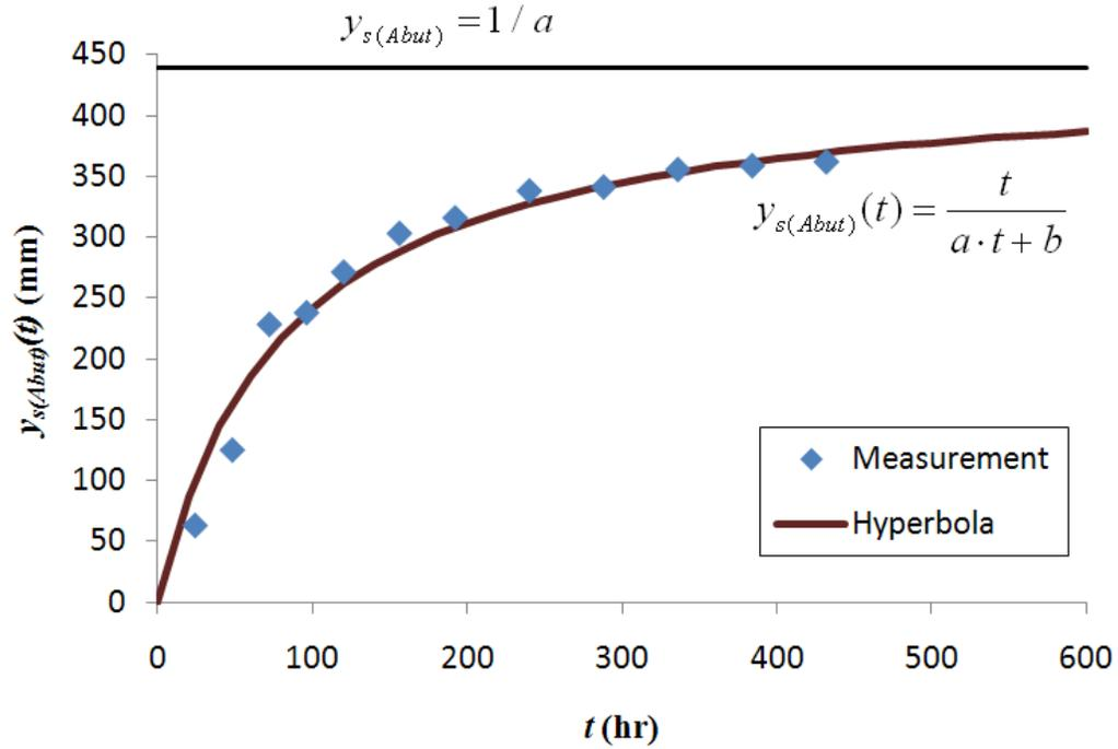
**Figure 23 – Abutment scour measurement and hyperbolic fit.**
