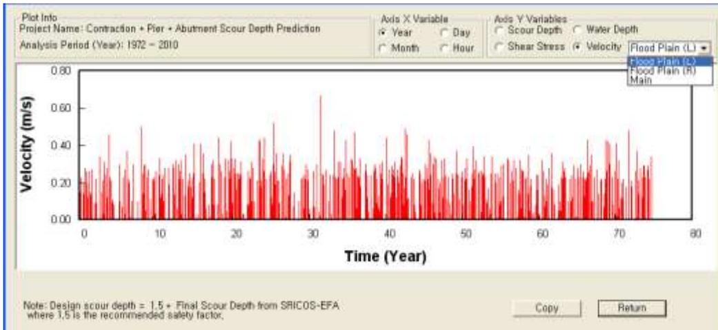
Figure 50 – Example of Output Plots (flow Velocity on Left Floodplain vs. Time).
