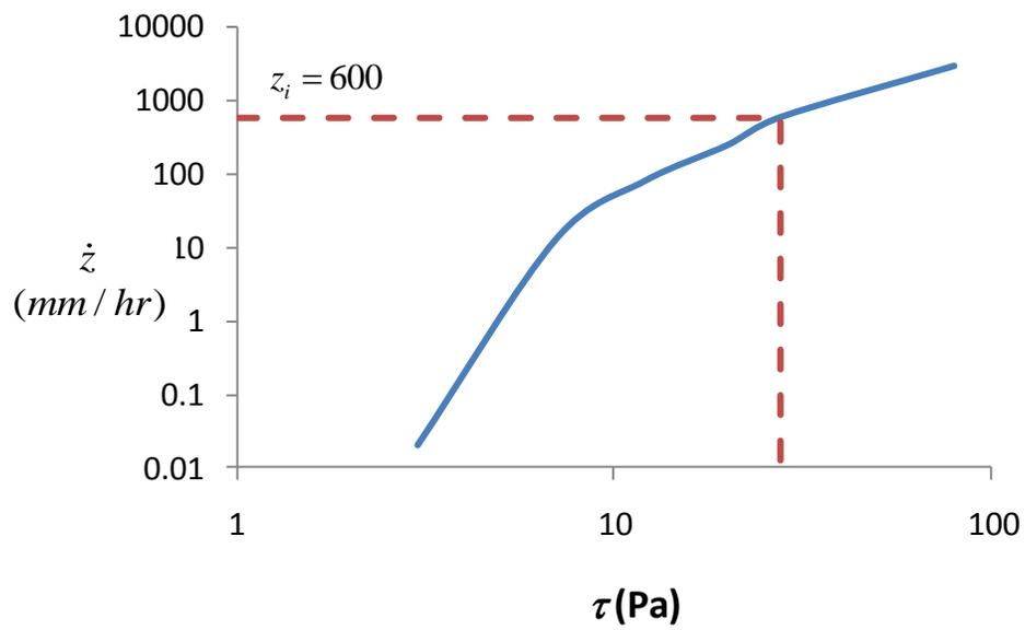
**Figure EX. 18 – Erosion function and initial erosion rate corresponding to the maximum velocity. (Example 5)**
