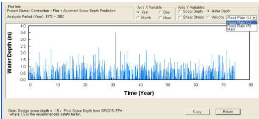
Figure 51 – Example of Output Plots (Water Depth on Left Floodplain vs. Time).
