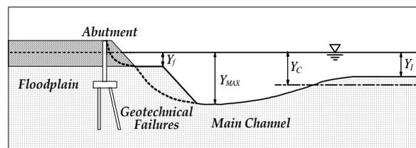
**Fig. 5** Short contraction scour as locally amplified contraction scour (Scour Condition A), and conceptual soil-failure surfaces
