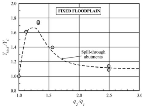
Fig. 11 Variation of  $Y_{MAX}/Y_C$  for wing-wall abutments on fixed floodplains subject to Scour Condition A
