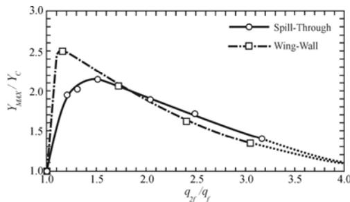
Fig. 12 Variations of flow-depth increase  $Y_{MAX}/Y_C$  against unit-discharge ratio,  $q_{2f}/q_f$ , scour Condition B
