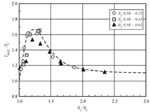
Fig. 8 Variation of  $Y_{MAX}/Y_C$  with  $q_2/q_1$  for Scour Condition A at spill-through abutments on fixed floodplains
