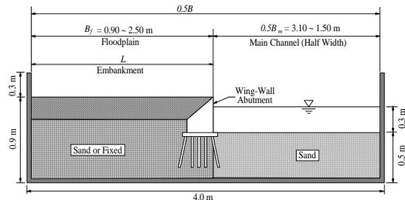
Fig. 10 Principal variables adjusted for wing-wall abutments subject to Scour Condition A
