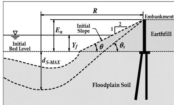
Fig. 3 Maximum scour depth is limited by embankment geotechnical stability (spill-through abutment)
