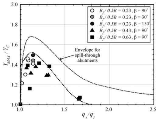
Fig. 9 Variation of  $Y_{MAX}/Y_C$  with  $q_2/q_1$  for Scour Condition A at spill-through abutments on erodible floodplains
