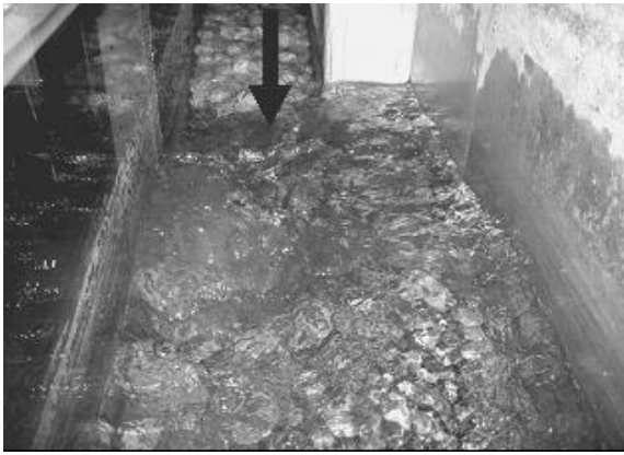
Fig.2 Plan view of an experimental test with B/b=1.67 (flow from upstream)
