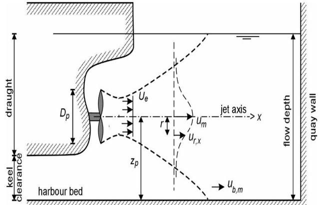
Fig. 3 Flow field behind a free propeller
