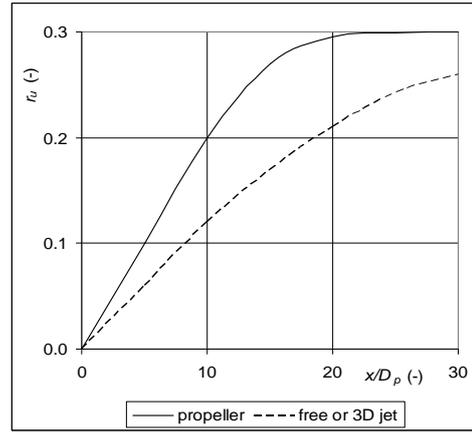
Fig. 2 Differences between turbulence of propeller and free jets
