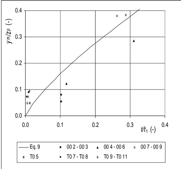
**Fig. 4** Time-dependent scour (Verheij 1983); to compute  $t_1$  in Eq. 9 the following assumptions are made: for sand  $U_c = 0.5$  m/s,  $U_u = u_{b,m}$ ,  $r_0 = 0.2$ ,  $\gamma = 0.8$  and  $\lambda = z_p$
