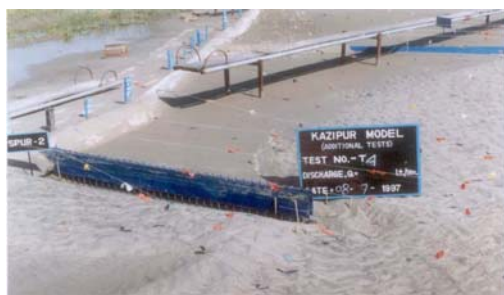
Fig.9 Scale model run showing a spur at Kazipur
