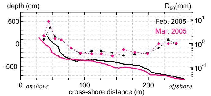
Fig.6 Comparisons of cross-shore bottom profiles &  $D_{50}$
